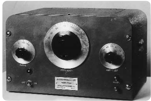
The 200A audio oscillator was Hewlett-Packard's first commercial success.
