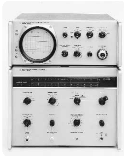
The 851A spectrum analyzer, with its wide sweep and tuning range, was a marvel of the early 1960s.
