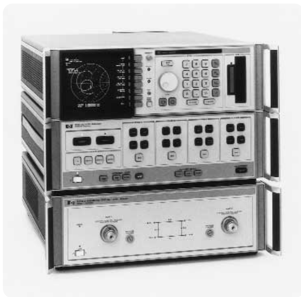
The 8510A network analyzer combined the power of microprocessors with extensive measurement capability to launch a revolution in component test.
