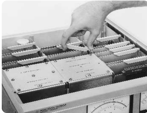
Modular printed circuit boards could be inserted and removed from the 8405A vector voltmeter for RF performance testing.
