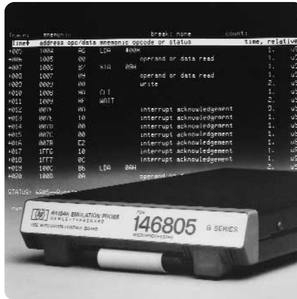
An emulator for the Motorola 146805G2 microcomputer added new capability to HP's 64000 logic development system.
