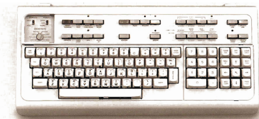
The terminal keyboard is marked with both APL and ASCII characters.
