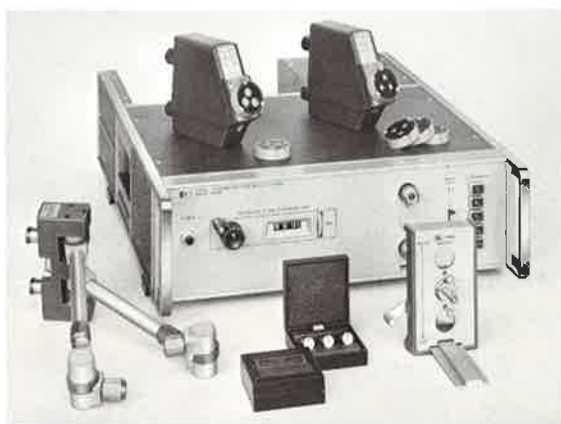
S-Parameter Test Set with device holding accessories
