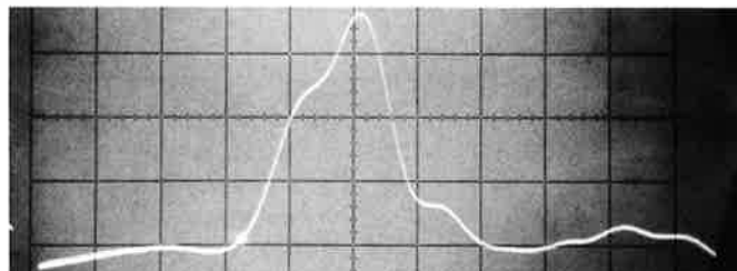
Magnified display of a BNC connector joining two 50-ohm cables. The horizontal axis is set at 2 cm/cm. Multiplying the 3.5 cm deflection by the reflection coefficient sensitivity of 0.01/cm, one can determine the connector has a \rho of 0.035.
