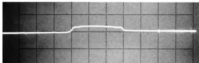
TDR display of a section of unknown cable spliced into a length of 50-ohm cable. Noting the distance setting of 40 cm/cm, and reflection coefficient sensitivity of 0.2/cm, one can determine the unknown cable is 120 cm long and has a Z_0 of 44 ohms.
