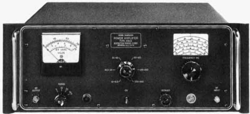
Figure 1. Type 230A Signal Generator Power Amplifier
