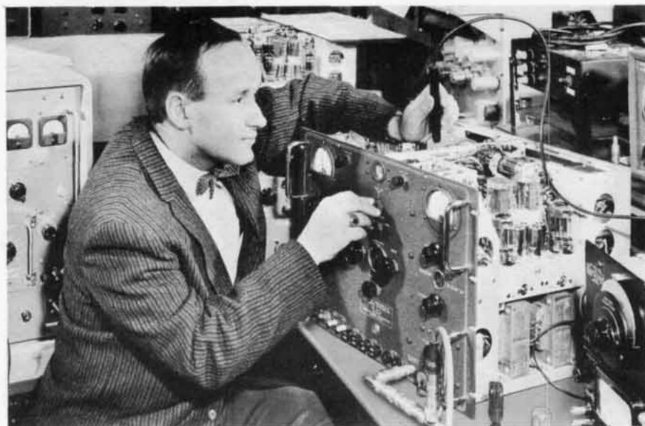
Figure 1. The author is shown final checking the RF tuning unit on one of the first production models of the TYPE 242-A FM Signal Generators.
