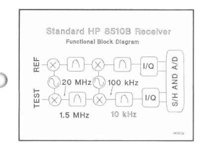
While Pulse Profiling could be possible with the standard HP8510, due to the low detector bandwidth, the pulse conditions needed to allow pulse profiling are not very useful.
