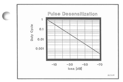
This chart shows the effect of pulse desensitization in loss of measurement dynamic range as a function of the pulse duty cycle. A duty cycle of 10% will cause a loss of dynamic range of 20 dB.
