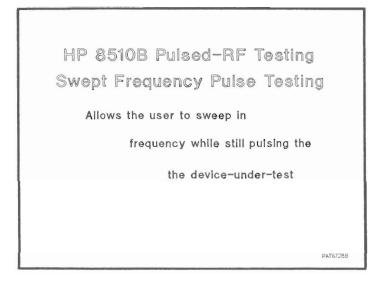
Swept Frequency Pulse testing shows the response of the DUT at a fixed point in the pulse as a function of frequency. This is a similar display to the traditional swept frequency measurement or to the Pulse Duty Cycle measurement. But with Swept Frequency Pulse testing, the data is NOT the CW or average pulse response but rather it is the response at a particular point in the pulse for range of frequencies.
