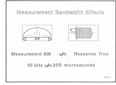
Given the limitation of a detector bandwidth of 10 kHz, it would be necessary to have a pulse width of greater than 200 microseconds with rise times of greater than 75 microseconds. So, to make useful Pulse Profiling measurements, the I.F. detector bandwidth needs to be increased.
