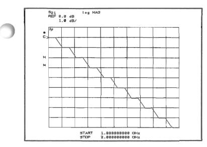
This is the measurement of a 10 dB step attenuator with two measurements at each attenuator level. Each measurement was made in response to an external trigger.
