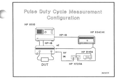
While the standard HP8510A/B can be used to do Pulse Duty Cycle, certain modifications to the measurement setup need to be made. In configuring the setup, a non-pulsed signal needs to be provided to the testset for phaselocking. It is injected into the a2 input via the rear panel coax link. An external modulator and pulse generator, such as the HP11720A and HP8116A, are used to create the pulsed-RF stimulus that is then applied to the testset via the normal RF IN port.
