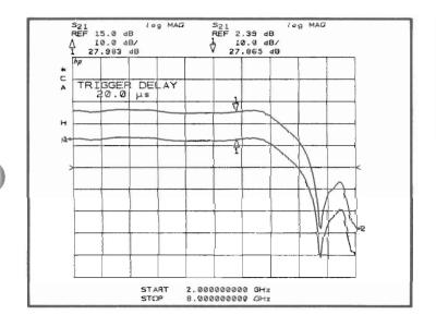
In the case of our DUT amplifier, there is little difference between normal Swept Frequency and Swept Frequency Pulse testing. This Swept Frequency Pulse measurement (upper trace) was with a 80 microseconds wide pulse measured 20 microseconds into the pulse.
