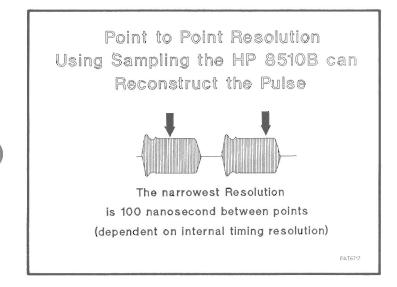
The HP8510 data conversion process is not fast enough to catch all the pulse data from a single pulse. Instead repetitive sampling is used where the data is reconstructed with samples taken from a series of pulses. A single data point is taken from each pulse with the delay time from start of the pulse progressively increased in as small as 100 nanosecond intervals.
