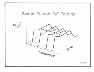
Swept Frequency Pulse testing is another way to view the 3-dimensional world of Response, Frequency and Time. In Swept Frequency Pulse the delay from start of pulse to the sample point is held constant and the response is viewed as a function of frequency. In Pulse Profiling, the frequency is held constant and the response is viewed as a function of time. If only we had a 3-D display!!
