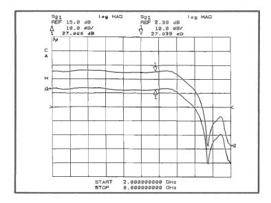
This measurement example compares the measurement of an amplifier under CW (upper trace) and Pulse Duty Cycle (lower trace) conditions (offset to better see the individual traces). In the Pulse Duty Cycle case the PRF was 100 kHz and the duty cycle was 50%. Note Error Correction is On and the results are nearly identical with perhaps a slight increase in the noise for the Pulse Duty Cycle case.
