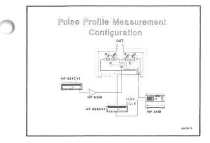
The HP85110A is fundamental mixer based testset designed for pulsed and high power DUTs. It looks much like a standard HP8510 system except for the additional HP8340/41 which provides the low noise LO. The HP8510B controls both sources using its multiple source capability. For pulsed-RF operation, the HP8510B provides a TTL output to drive the RF source internal pulse modulator.
