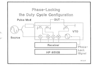
This detailed block diagram shows how the non-pulsed-RF is used by the testset and receiver for a phaselock reference. The other samplers and DUT measure the modulated pulsed-RF waveform.
