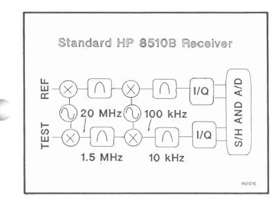
This functional block diagram will help explain how the standard HP8510 LF. chain will react to a pulsed-RF waveform. The TEST and REFERENCE signals are first downconverted to 20 MHz in the testset with roughly 1.5 MHz of bandwidth. A second conversion occurs to 100 kHz followed by a synchronous detector (I/Q) with a bandwidth of 10kHz.
