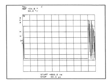
This is the phase response of the previous measurement. Note: outside the pulse (before 0 microseconds and after 35 microseconds) there is no signal and therefore the response is just noise.
