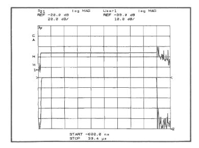
This is an example of the pulse profiling measuring capability. Shown is the S21 and the unratioed output power of our amplifier tested with a 35 microsecond pulse at 4 GHz. The S21 measurement as function of time is fully error corrected and the system has absolute accuracy specifications, both capabilities not found in previous systems.
