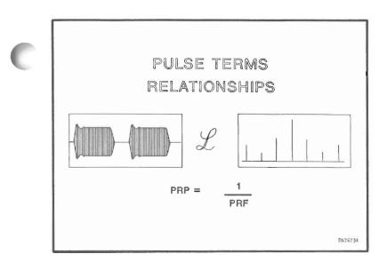
The pulsed-RF waveform can be viewed in either the time domain or the frequency domain. One fully describes the other, and the choice depends which is more convenient to observe a particular characteristic.
