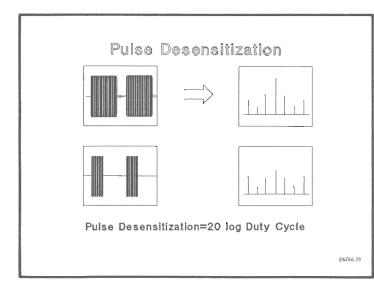
As explained earlier, a pulsed-RF waveform consist of central and additional spectral lines, and in the Pulse Duty Cycle case, only the central line is detected. As the duty cycle decreases, the total energy in the central line decreases. This causes an overall decrease in detector dynamic range and is called Pulse Desensitization.
