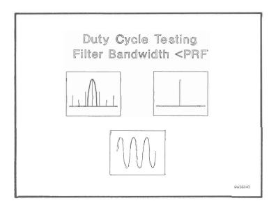
Let's first study the case where the pulse's PRF is much greater than the detector's bandwidth. This mode will be called Pulse Duty Cycle.
