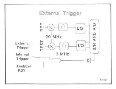
The external trigger is a TTL input on the rear panel of the HP8510B. It is edge triggered and will be ignored if the analyzer is not yet ready to be triggered. The Analyzer RDY signal is also available on the rear panel (Stop Sweep) for the user. The external trigger is usable with both detectors. In case of the wide bandwidth detectors, there is an user adjustable trigger delay. External trigger is particularly useful in pulse testing, when a particular duty cycle or PRF is desired.
