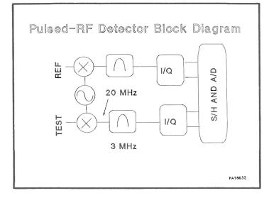
The HP8510B Option 008 provides new detectors with improved bandwidth permitting usable pulse widths as small as 1 microsecond. This allows the testing of DUT under actual operational conditions without the harmful heating effects and is even fast enough to view some transient behavior.
