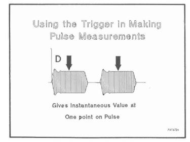
Like in the Pulse Profiling measurement, a single data point is taken on a pulse, but instead of increasing the time delay, the time delay is fixed and the carrier frequency for the next measurement is changed. The value of the delay is user adjustable in 100 nanosecond intervals.
