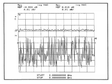
This measurement example shows the effects of pulse desensitization in the case of 10% duty cycle (lower trace) compared to a 100% duty cycle (CW -- upper trace). Only at these very high amplitude resolutions can the increase in noise be seen.
