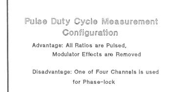
All measurements are made as ratios of pulsed-RF signals, and all modulator effects (loss and phase shift) are removed. However, with the testset reconfiguration, the S-parameter testset has been converted into a Reflection / Transmission (R/T) testset. This means that to obtain all four S-Parameters, the DUT will have to be manually reversed.
