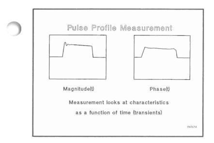
With the ability to profile the pulse envelope, one can view both the magnitude and phase response as a function of time. This means under pulsed (non-CW) conditions certain DUT characteristics can be observed, such as the droop or change in the response due to DUT heating or power supply capacity limitations.
