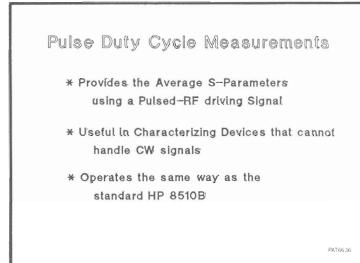
Pulsed Duty Cycle operation measures the average response of the DUT to a pulsed-RF waveform and cannot show the response at a particular point in time of the pulsed-RF stimulus. This is still very useful for testing DUTs that are unable to handle CW stimulus and the behavior during the pulse is constant. Typical uses would be for testing transistors or MMICs on wafer before packaging.
