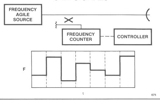
Many modern transmitters (and therefore LO's and spot jammers) use frequency agility. The frequency counter's wide instantaneous bandwidth allows for up to 1200 MHz at baseband and 50 MHz deviation to 50 GHz (heterodyned).
