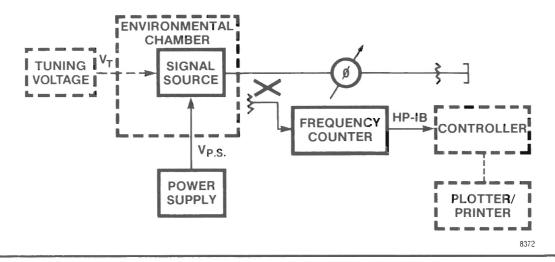
The frequency drift, stability, modulation sensitivity, pulling and pushing figures, and synthesizer frequency setting may be easily measured with a low cost frequency counter.
