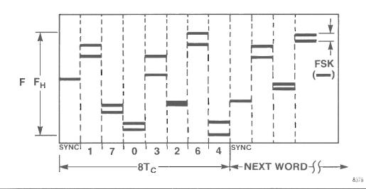
M-ARY Frequency Shift Keying (MFSK) message modulation and frequency hopping diversity communication systems require the measurement of frequency during the data bit period Tc to determine proper frequency transmission according to shift keying and hopping deviations.
