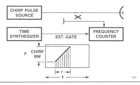
A radar chirp pulse frequency measurement is made by moving an external gating signal successively across the chirp pulse width. For chirp radar applications the modulation accuracy is paramount, while doppler radars require minimal FM on the burst.
