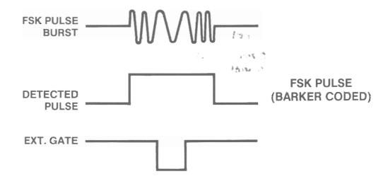
By positioning an external gate to the region of interest, the pulse frequency from the group, or the FSK pulse frequency modulation can be measured.
