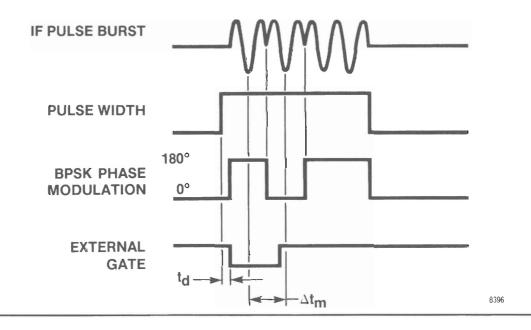
By arming the time interval measurement of the counter, in the same manner as for MPSK signals, the phase coded modulation can be measured. Varying the time delay from the start of the pulse and external gate width would enable demodulation analysis of the phase coded radar
