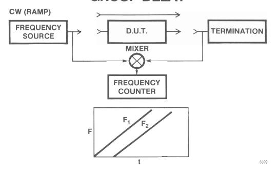
$$\begin{aligned} & F_1 = kt \\ & F_2 = k(t + \tau_{\phi}) \\ & F_1 \text{-} F_2 = k \; \tau_{\phi} = k \frac{\phi_1}{\omega_1} \\ & \tau_g \cong \frac{\Delta \phi}{\Delta \omega} \cong \frac{\Delta \; (F_1 \text{-} F_2)}{k} \; \text{for short gate times} \end{aligned}$$
