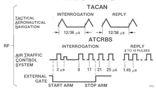
Precision time measurements may be made of complex pulse timing by externally gating the time counter. For example, the 21  $\mu$ sec delay of the ATCRBS interrogation signal can be measured if the external gate signal is applied as shown.
