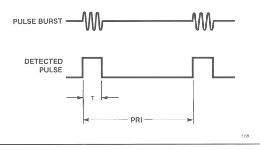
Modern microwave frequency and time counters measure the pulse burst frequency, the pulse width, and PRI or PRF of radar signals.
