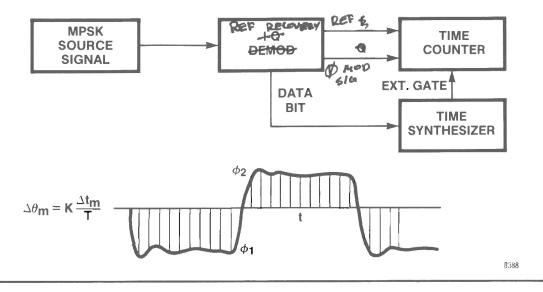
By gating the time counter with successive gate widths the time interval transient can be profiled in the same manner the step tuning transient or chirp pulse was measured.
