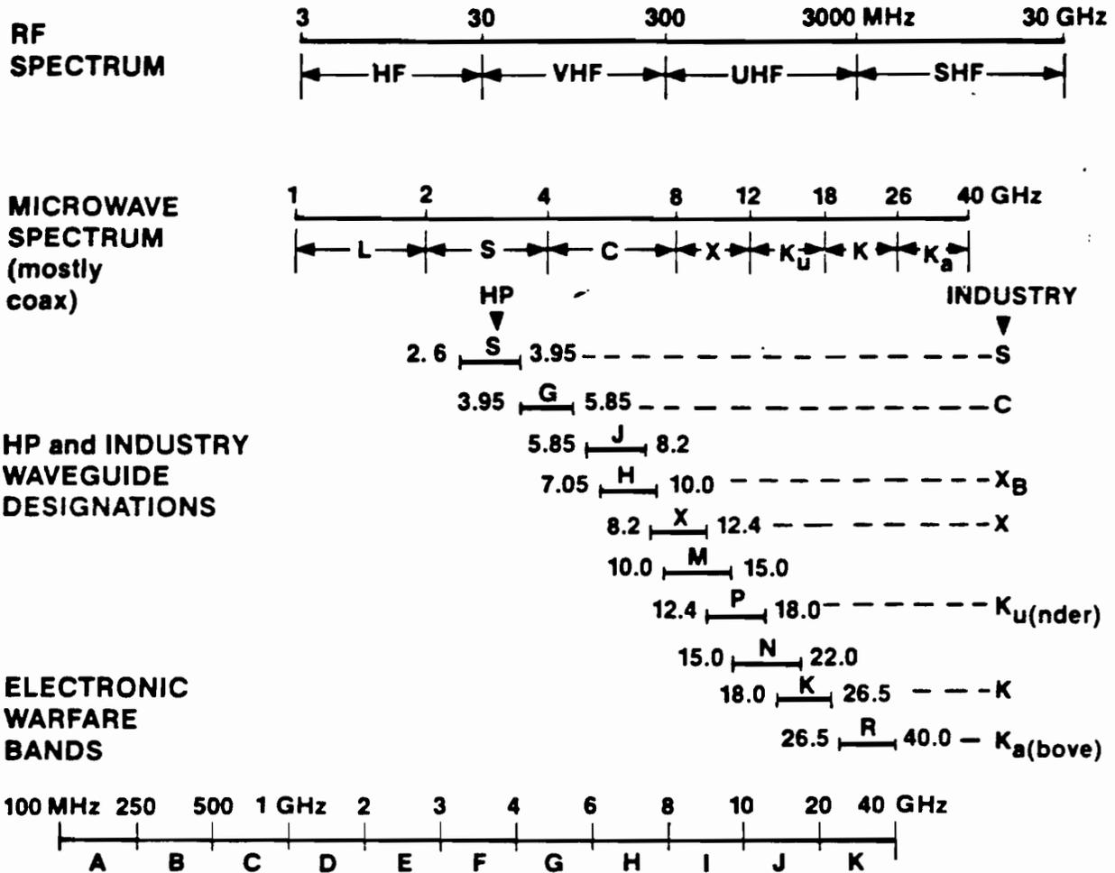
The term *microwaves* is commonly understood to range from about 300 MHz (1 meter wavelength) to above 300 GHz (1 mm wavelength). By far most activity is below 18 GHz with some emerging communication, radar, and EW usage going to 40 GHz and a little radar work to 100 GHz and beyond.
