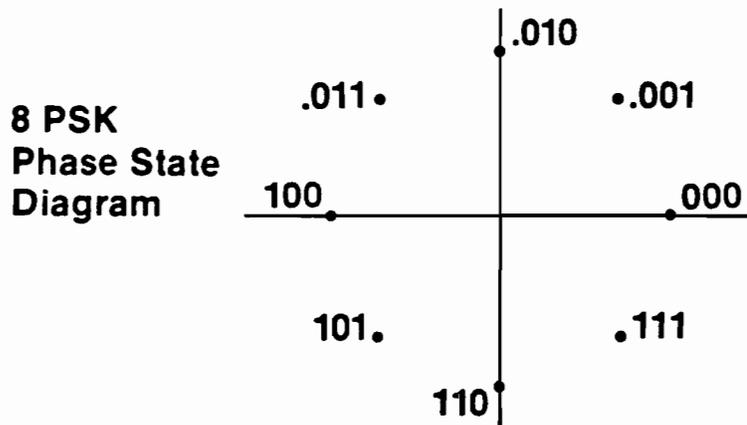
A typical transmitter for a Time Division Multiplex system uses the same RF elements that we saw earlier for the Frequency Division Multiplex system, but phase modulates the 70 MHz local oscillator. The data stream from the digitized 24 voice channels changes the phase between 2, 4 or 8 states. The polar diagram shows the phase states on an 8 PSK system where each state represents 3 bits in the data stream.
