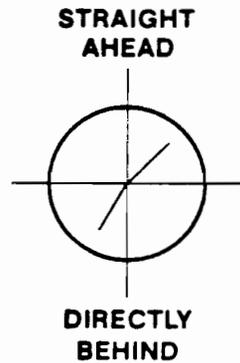
Shows pilot bearing of radar transmitter that matches signature of known enemy equipment. Here we see threats at 1:00 and 7:00 o'clock.
