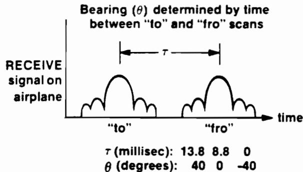
Let's take a look at how one of these navigation systems (MLS) operates. It's referred to as a time reference scanning beam system (TRSB). This system uses an electronically steered antenna array that transmits a well defined beam over a sector of  $40^\circ$  either side of the runway. It scans that sector in a precisely timed manner so that the difference in time between successive scans tells the receiver on board the airplane what its bearing is with respect to the center line of the runway.
