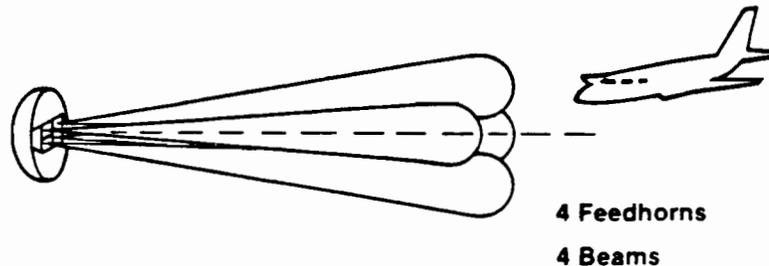
**Return signal phase front is processed with sum and difference hybrids to compute angle off boresight from single pulse**
