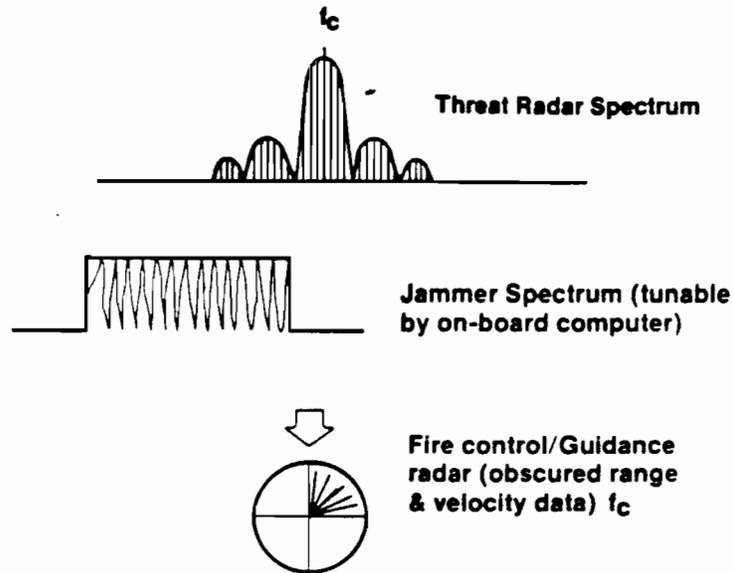
Jamming can be noise or deception jamming. If you can get enough noise into the other receiver, it might "break lock". Or you can retransmit slightly modified versions of the threat signal to make it look like your aircraft is moving way from where it really is. ECM transmitters are multi-band dual-mode (pulse and CW) moderate power TWT (500-1000 watts), often mounted in external pods.
