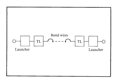
The most satisfactory approach is to model the discontinuities and then to de-embed the device under test from a measurement made at the test port connectors based on a highly reliable calibration scheme based on repeatable components with precision connectors.
