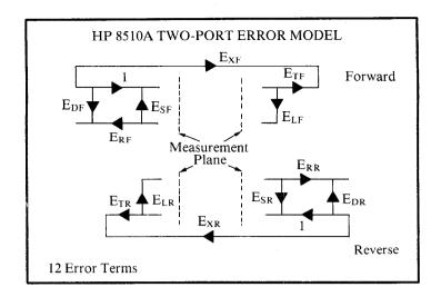
As discussed above, this approach is quite straightforward for simple cascades (no matter how many components or ports are involved but becomes more complicated when there are inter-port couplings. This is illustrated in the slide which shows the two-port (12-term) error model used by the HP 8510. If there are any additional inter-port couplings associated with the devices connected between the measurement planes, the strategy described earlier will break down.
