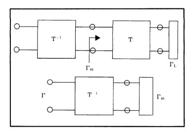
We can then obtain  $\Gamma_m$  in terms of  $\Gamma_L$  . However if the network is now cascaded with the inverse T-matrix, we obtain automatically  $\Gamma_L$  in terms of  $\Gamma_m$  .
