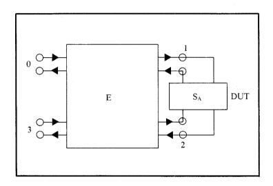
The generic solution for the two-port DUT is to use a four-port network to model the error adapters at both ports and the inter-port couplings. The essence of the arrangement is shown in the diagram; ports 0 and 3 are the measurement ports, the two-port device under test  $(\mathbf{S}_{A})$  is connected between ports 1 and 2.
