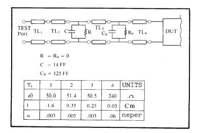
All transmission lines are specified in terms of  $Z_0$ , length and loss (assumed small but non-zero).
