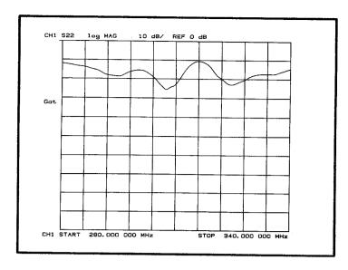
The frequency response of the signal reflected at time t=0 is more independent of frequency but shows variation due to the tuning inductors and the acoustic impedance of the transducer.
