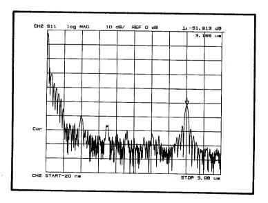
Transforming S11 frequency data to the time domain can give yet more insight into the operation of the filter. Here the main response is due to electrical reflections at the launching IDT. Marker 1 is placed on the main peak of the signal which was reflected from the receiving IDT at 3.188 us. Again, other spurious reflections can be observed in the region between the single and double transit signals.
