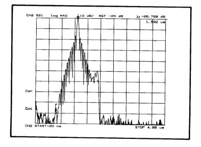
Another powerful feature of the HP 8753A is the time domain gating capability. This capability allows the user to gate out the spurious time signals in order to determine the filters frequency response without the interfering spurious signals. By placing the gate center at the peak of the time response and adjusting the gate span to include all of the filter sidelobes, we can perform an inverse transform of the gated data to obtain the idealized frequency response.
