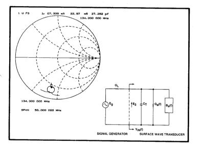
Measurement of S11 allows quick determination of the IDT radiation conductance and capacitance. The marker can be set to display impedance or admittance. In this case, admittance is dispayed. The value of capacitance or inductance is also computed and displayed. This allows equivalent circuit parameters to be measured at a glance.
