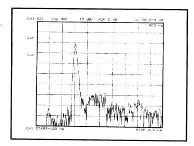
Here we use the time domain gating features of the 8753A to remove the effects of feedthrough to simulate performance in a properly shielded circuit board application.
