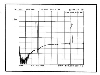
A response at three times the fundamental frequency is also observed in this particular filter. This response is produced by the inherent spatial asymmetry of the electric field produced by the split finger IDT's commonly used in brickwall filters.
