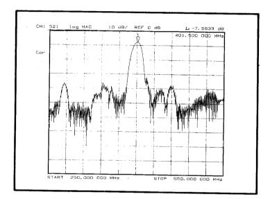
Shown here is the response of a group-type SAW filter with passband at 400 MHz. The passband minimum insertion loss is seen to be about 7.6 dB. Feedthrough is clearly visible at the 40 - 60 dB level below the input. Much of this feedthrough is test-fixture related, and will be eliminated in a properly shielded circuit board application.
