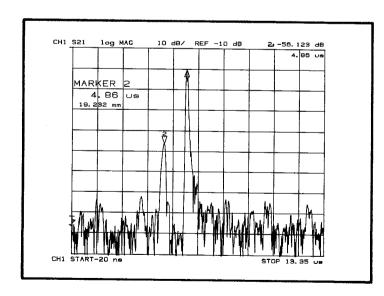
Here we show the transform using 801 points. The triple transit signal occurs, incorrectly, before the single transit signal due to aliasing. Instead of employing more points, aliasing can be eliminated by reducing the frequency span of the original measurement.
