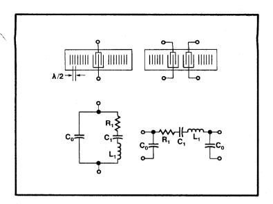
Within a few hundred kilohertz of the center frequency, this device can be modeled as a series resonant circuit. Note that both 1-port and 2-port resonator configurations are possible. The 2-port configuration is usually preferable because of the high isolation out-of-band between input and output ports. The 1-port model is the same as that for a bulk crystal resonator.
