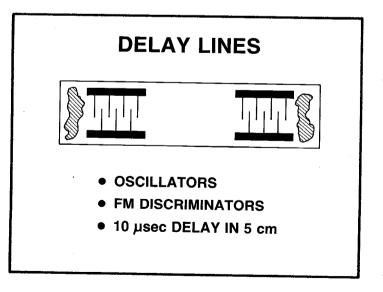
Low propagation loss for SAWs in crystals makes possible compact, convenient delay lines of 10 usec or more delay. These are highly useful in oscillator control, in FM discriminators, and other applications. The HP 8753 network analyser can be used to measure important characteristics of SAW delay lines in both the frequency domain and the time domain.
