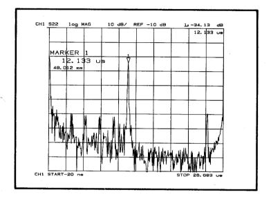
The transform of the S22 data reveals both a double and quadruple transit signal. Due to the long time span, 1601 points are required for this transform.
