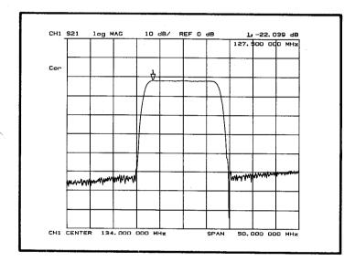
The frequency response of a typical brickwall filter is shown in this figure. In order to improve the dynamic range of the instrument, the IF bandwidth was reduced to 30 Hz. Marker 1, positioned at the peak of the response, shows a minimum insertion loss of 22.04 dB. The stopband rejection can be seen to be about 50 dBc.
