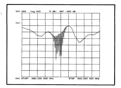
Reflected signals returning to the sending transducer are also easily measured on the HP 8753A. This figure shows S22 for a signal injected at the apodized transducer and reflecting from the unapodized transducer. The ripples indicate interference between an electrically reflected signal and an acoustically delayed signal.
