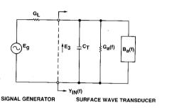
Where:  $C_T$  = static IDT capacitance
