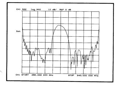
Transforming the double transit signal gives a frequency response response dominated by the filter apodization.
