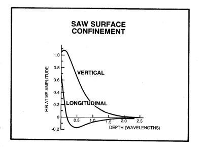
The free surface of a crystalline solid provides a natural waveguide for SAWs. The amplitude decays exponentially into the interior of the substrate for both the vertical and longitudinal components of the motion. Note that most of the energy is trapped within 1 wavelength of the surface [4,5]. This has the great advantage of access to signal processing elements which can be fabricated easily on the exposed surface.
