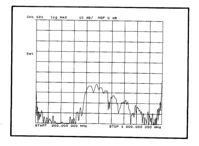
The frequency response of the two most dominant time responses is shown here. These responses account for most of the bulk mode energy that is launched in this device. Fortunately, these waves do not contain appreciable energy at the SAW frequency, but they do affect the far out stop band rejection. Without using the black wax absorber, these waves could not be observed in the presence of the stronger SAW response.
