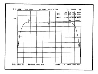
The 40 dB bandwidth, of 19.07 MHz, is just as easily obtained using the marker width search feature. The shape factor can now be computed as the ratio of the 40 dB bandwidth to the 3 dB bandwidth which gives a shape factor of 1.23 for this filter. Such a shape factor is routinely achievable with SAW filters due to their transversal character [4,5].
