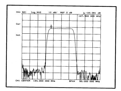
The gated frequency response shows improved stopband rejection due mostly to reduced electromagnetic feedthough as a result of the gating. Now the acoustic sidelobes are readily observed in the response.
