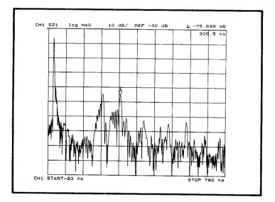
Each response corresponds to a different bulk wave or a multiple bounce of one of the waves. Note that one of the stronger responses has a time delay which is close to the SAW delay of 320 ns. This could be a potential source of frequency response degradation, especially if this energy is launched close to the SAW frequency. To see the frequency content, the user can place the gate around the time response of interest and transform back to the frequency domain.
