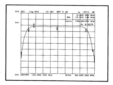
This figure shows the filter passband. Here marker 1 has been zeroed so that the marker width search feature can be used to determine the 3 dB bandwidth. Markers 3 and 4 are positioned at points 3 dB lower than marker 1. The user can immediately read the 3 dB bandwidth which is 15.51 MHz. The center frequency of the filter has also been computed as the average of the 3 dB frequencies and can be seen to be 133.83 MHz.
