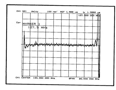
This figure shows the group delay over the passband region. The group delay is a measurement of the time delay of the filter as a function of frequency. Deviation of the group delay from a constant value over the passband region can lead to signal distortion since different frequency components are delayed by different amounts. This is especially important for broadband filters.
