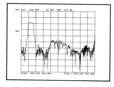
This plot shows a wide sweep of an in-line Brickwall filter. This device has a center frequency of about 300 MHz and a time delay of about 320 ns. The bulk mode spurious response can be seen in the region around 600 MHz. Most of the bulk modes are launched at frequencies higher than the SAW frequency. In fact, most of the energy is launched at about twice the frequency of the SAW.
