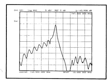
A simple, coaxial two-port fixture is used here to measure the transmission response of a SAW resonator centered at 742.5 MHz. A single thru-line calibration was done to remove the losses of the fixture and cables using the "RESPONSE" option in the calibration menu. Measuring the log of the magnitude of S21 shows good agreement with the modeled response above.
