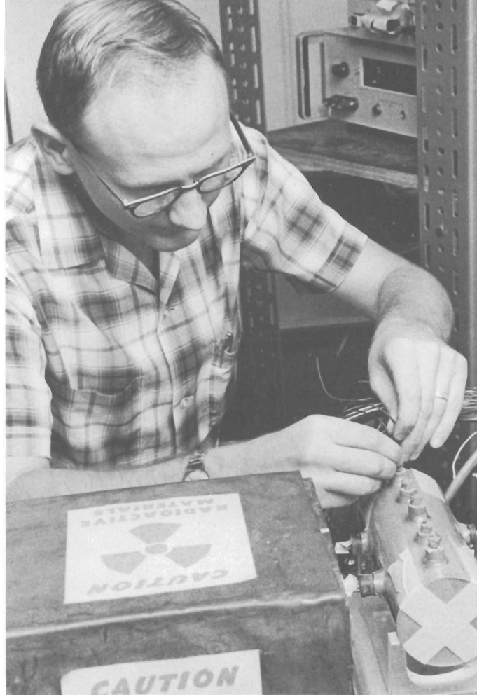
Hydroscience project involving gamma rays to measure the movement of water in soil sample is conducted by Keith Cassel in Davis soil water sciences laboratory. Harrison Division power supply unit is used in test. Many field tests are also conducted on 4,000-acre campus. Everett LaRue, a graduate student, checks gauges used in soil-water flux tests. Hundreds of such instruments are linked to a recording and computer center to provide comprehensive data on complex interaction of water, soil, crops, heat, and additives.
