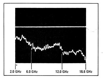
Figure 3-5. Unleveled RF Power Output for Sequential Sweep
