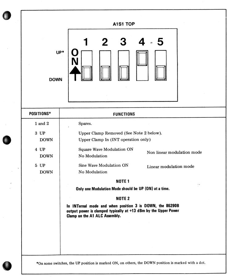
Figure 3-12. Switch Positions and Functions for ALC Function Switch A1S1
