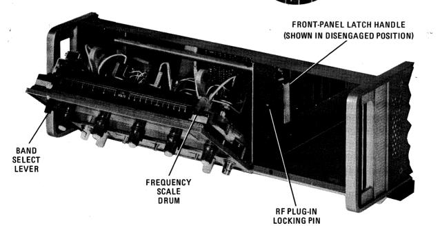
Figure 2-1. Location of Mainframe Parts Pertinent to Frequency Scale and RF Plug-in Installation
