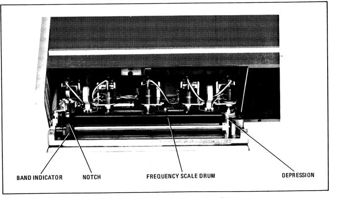
Figure 2-2. Mainframe Front Panel in Open Position
