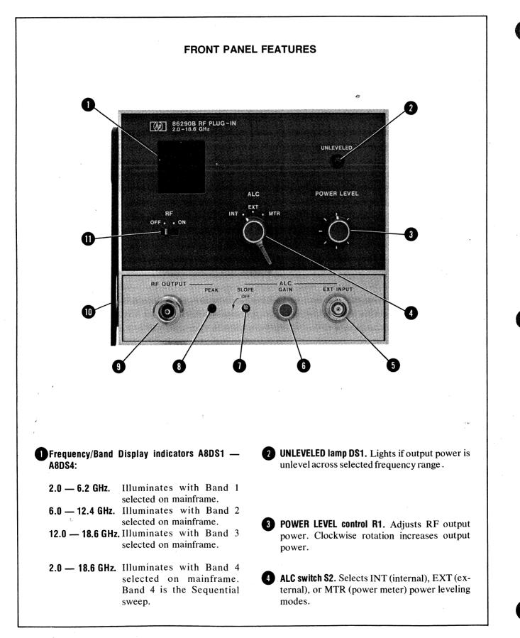
Figure 3-2. Front Panel Controls, Connectors and Indicators (1 of 4)
