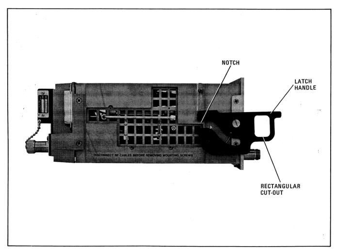
Figure 2-3. RF Plug-In Latch in Release Position
