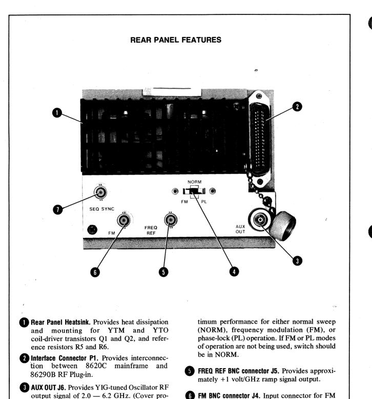
vided should be installed when AUX OUT not used.)
