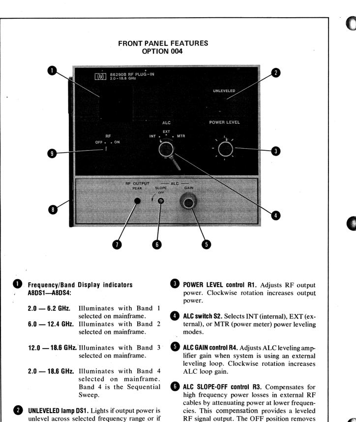
Figure 3-2. Front Panel Controls, Connectors and Indicators (3 of 4). Option 004
