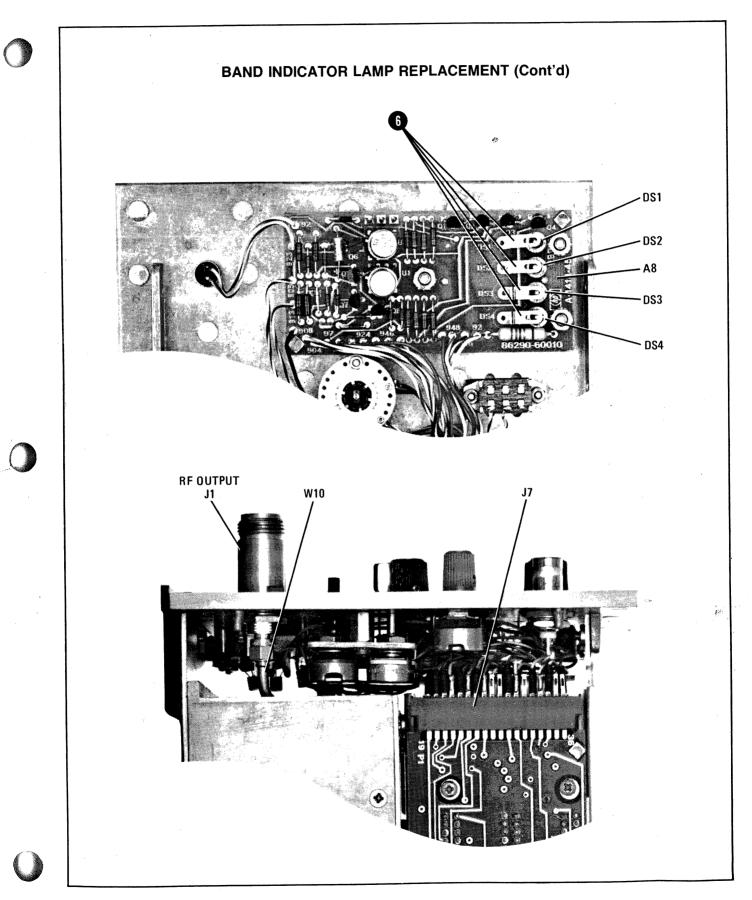
Figure 3-13. Band Indicator Lamp Replacement (2 of 2)
