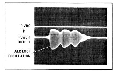
Figure 3-9. Oscillations Due to Excessive ALC Loop Gain
