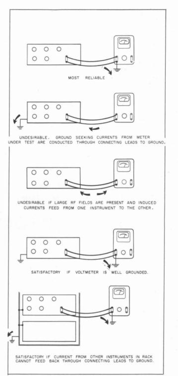
Figure 2-2. Desirable and undesirable arrangements for grounding instrument chassis when using the Voltmeter Calibration Generator The accuracy of the 738A is determined by:
