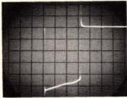
A. Test Points 31-33 5 \mu sec/cm, 5v/cm
