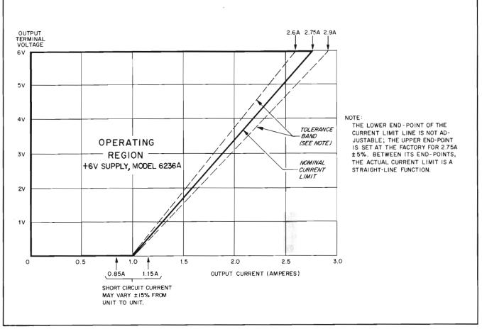
Figure 3-3. Current Limit Characteristics of the 6V Supply (Model 6236A)
