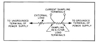
Figure 5-2. Current Sampling Resistor Connections
