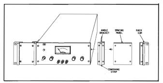
Figure 2-2. Rack Mounting, One Unit
