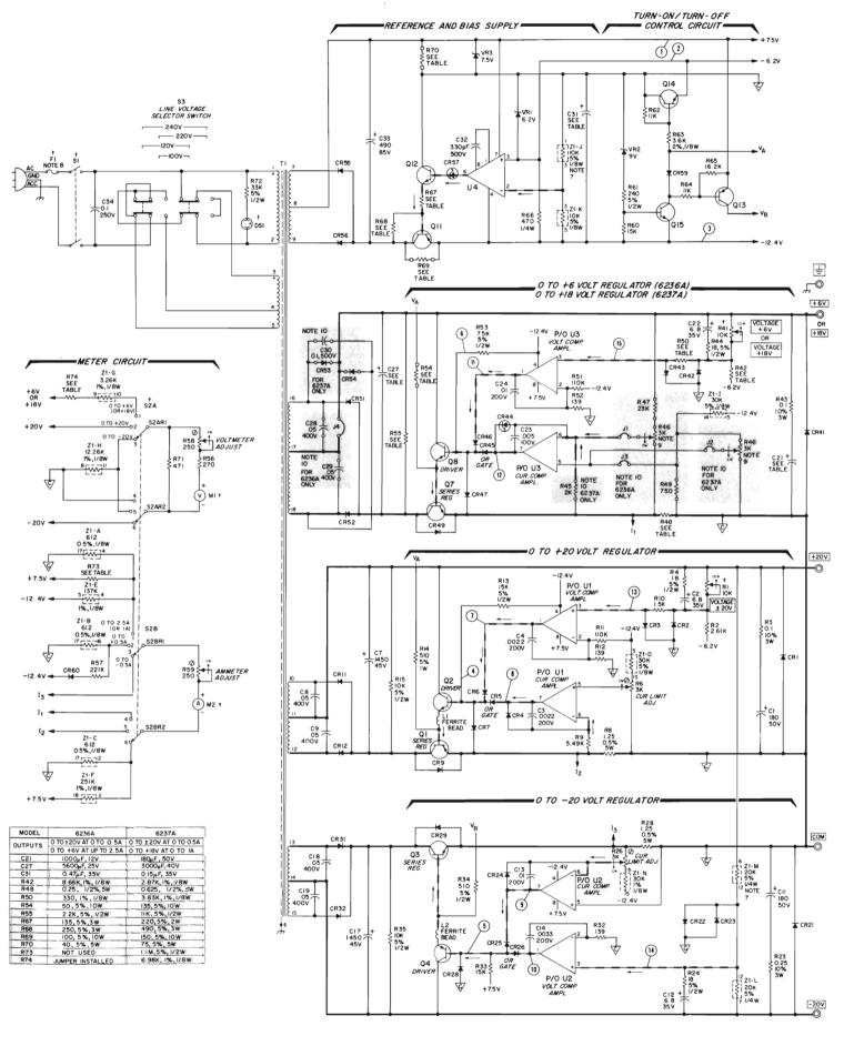
Figure 7-1. Models 6236A and 6237A, Schematic Diagram
