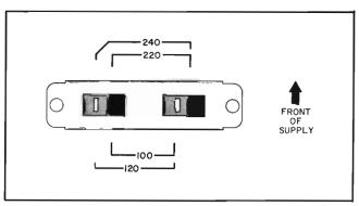
Figure 3-2. Line Voltage Selector (Set for 120 Vac)
