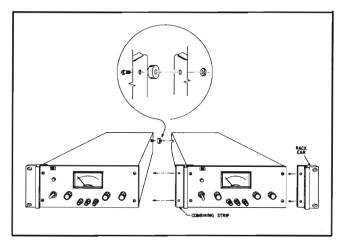
Figure 2-3. Rack Mounting, Two Units
