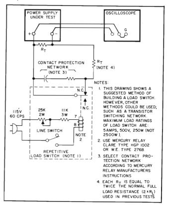
Figure 5-5. Load Transient Recovery Time, Test Setup
