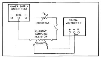
Figure 5-3. Output Current, Test Setup
