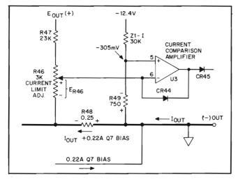
Figure 4-1. Foldback Current Limit Circuit in 6V Supply
