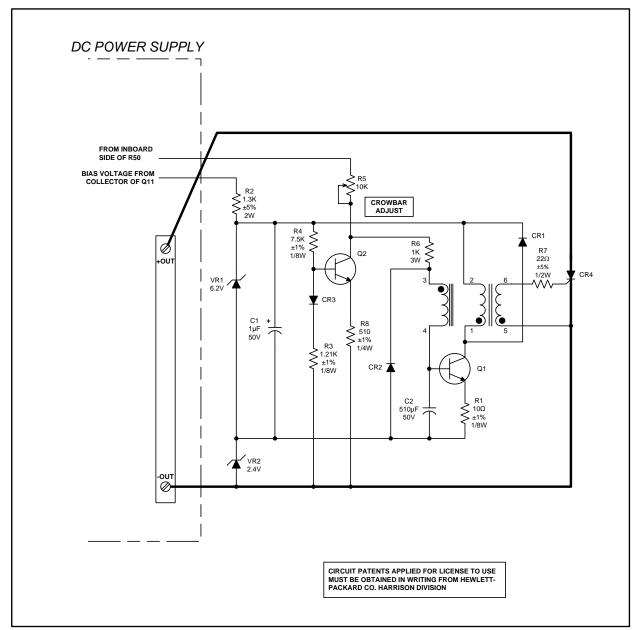
Figure A-1. Model 6101A and 6111A Overvoltage Protection Crowbar
