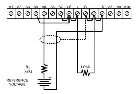
Figure 3-4. Remote Voltage Programming (Constant Voltage)
