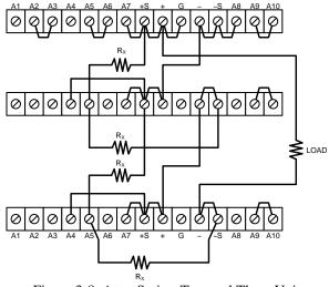
Figure 3-8. Auto-Series, Two and Three Units
