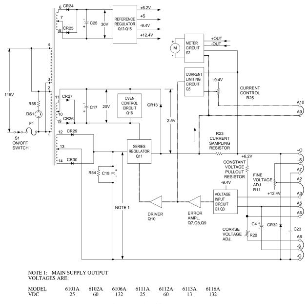
Figure 4-2. Simplified Schematic
