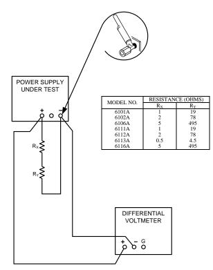
Figure 5-5. Load Regulation, Test Setup
