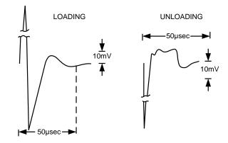
Figure 5-8. Transient Recovery Time, Waveforms
