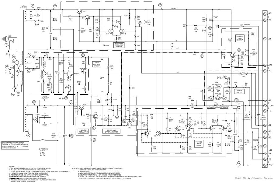
Model 6101A, Schematic Diagram
