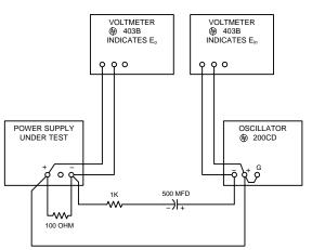
Figure 5-9. Output Impedance, Test Setup
