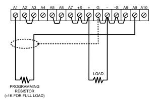
Figure 3-5. Remote Resistance Programming (Current Limit)
