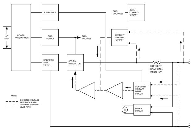
Figure 4-1. Overall Block Diagram
