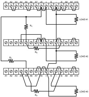
Figure 3-10. Auto-Tracking. Two and Three Units
