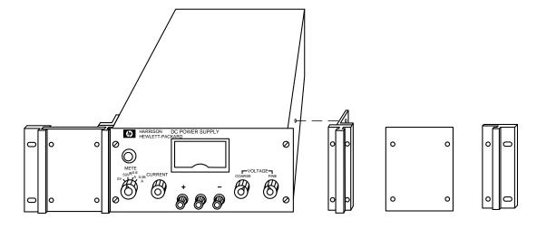
Figure 2-3. Rack Mounting, One Unit
