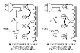
Figure 2-1. Input Transformer Primary Connections
