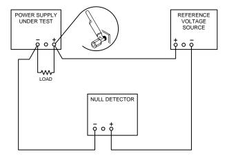
Figure 5-3. Differential Voltmeter Substitute Test Setup
