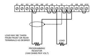
Figure 3-3. Remote Resistance Programming (Constant Voltage)
