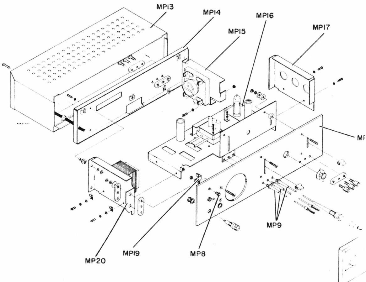
Figure 6-2. Location of Mechanical Parts, Rack Model
