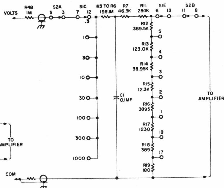
Figure 5-8. Simplified Schematic, Voltmeter Switching
