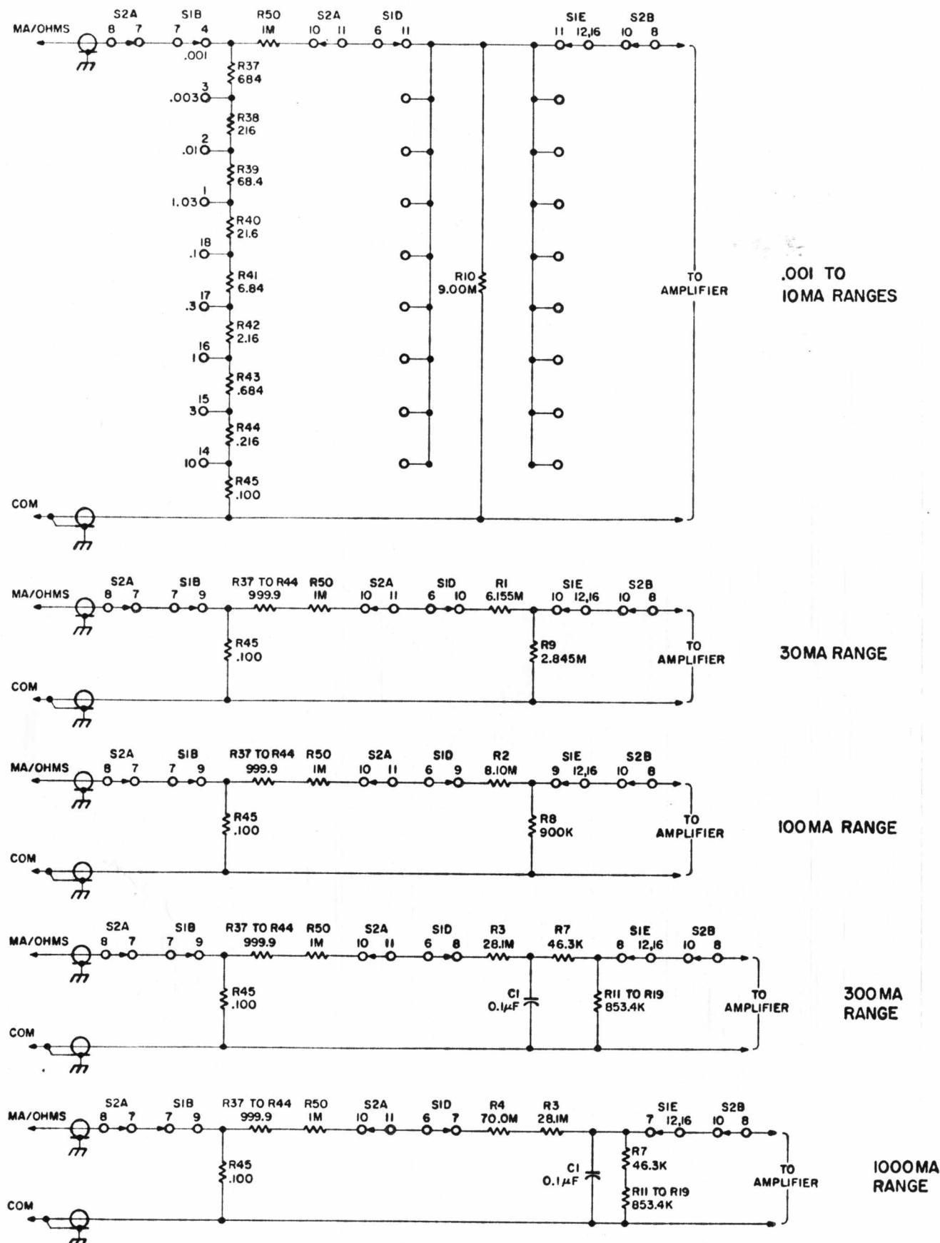
Figure 5-9. Simplified Schematic, Ammeter Switching
