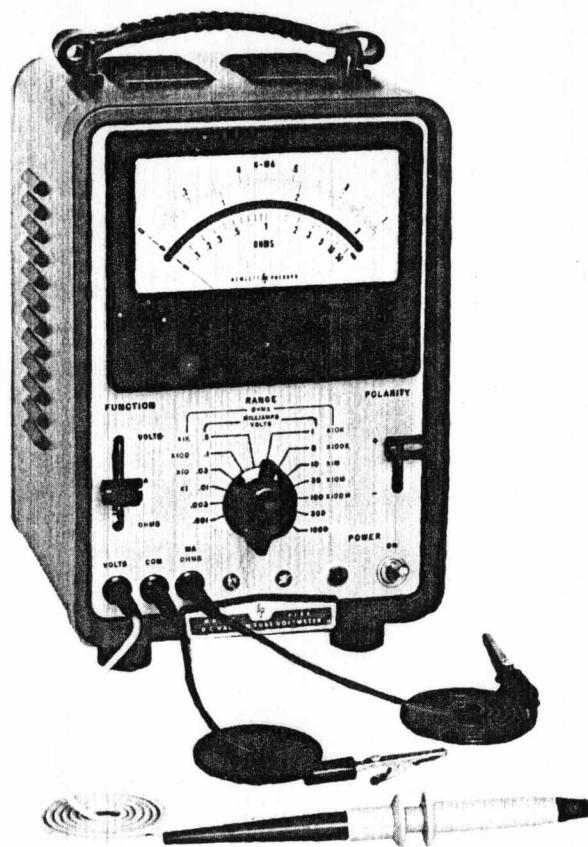
Figure 1-1. Model 412A DC Vacuum Tube Voltmeter
