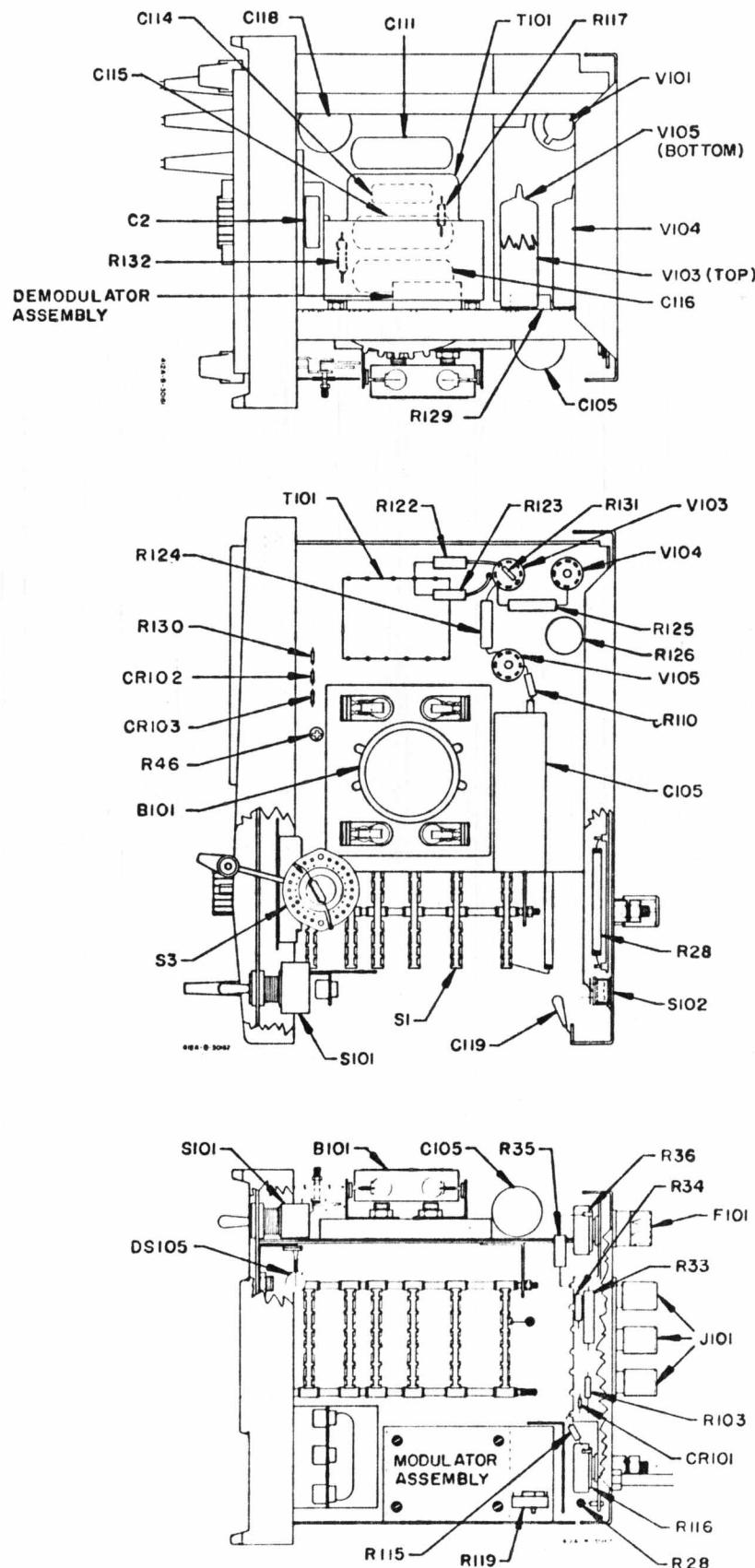
Figure 7-1. Location of Chassis Mounted Parts, Cabinet Model
