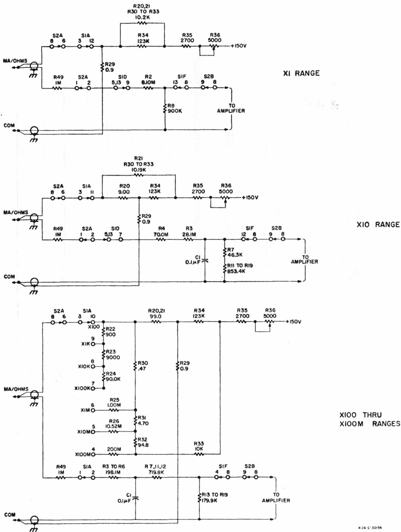
Figure 5-10. Simplified Schematic, Ohmmeter Switching
