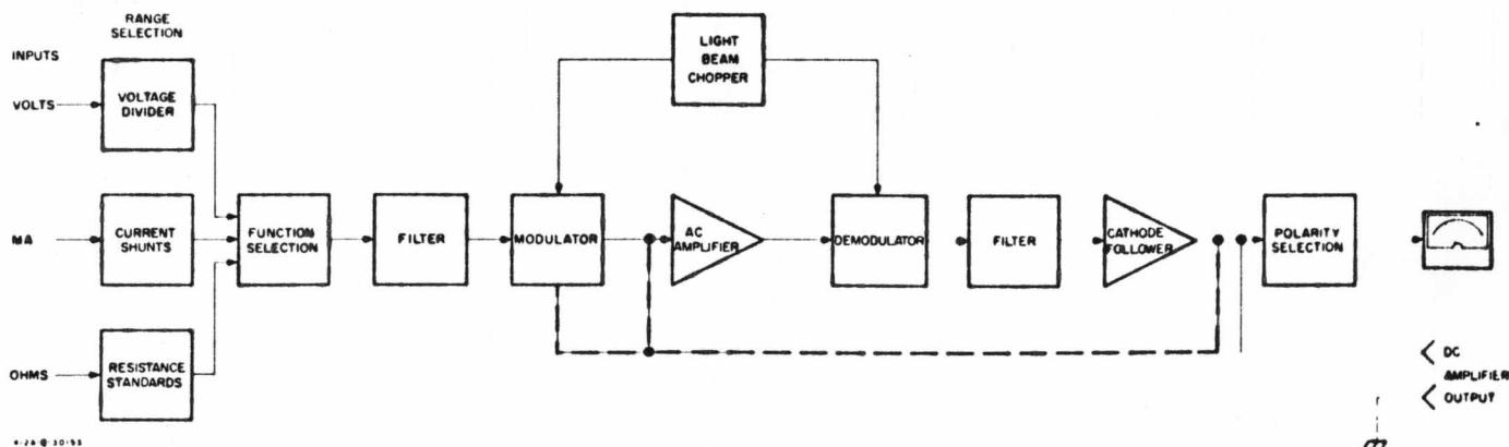
Figure 4-1. Block Diagram
