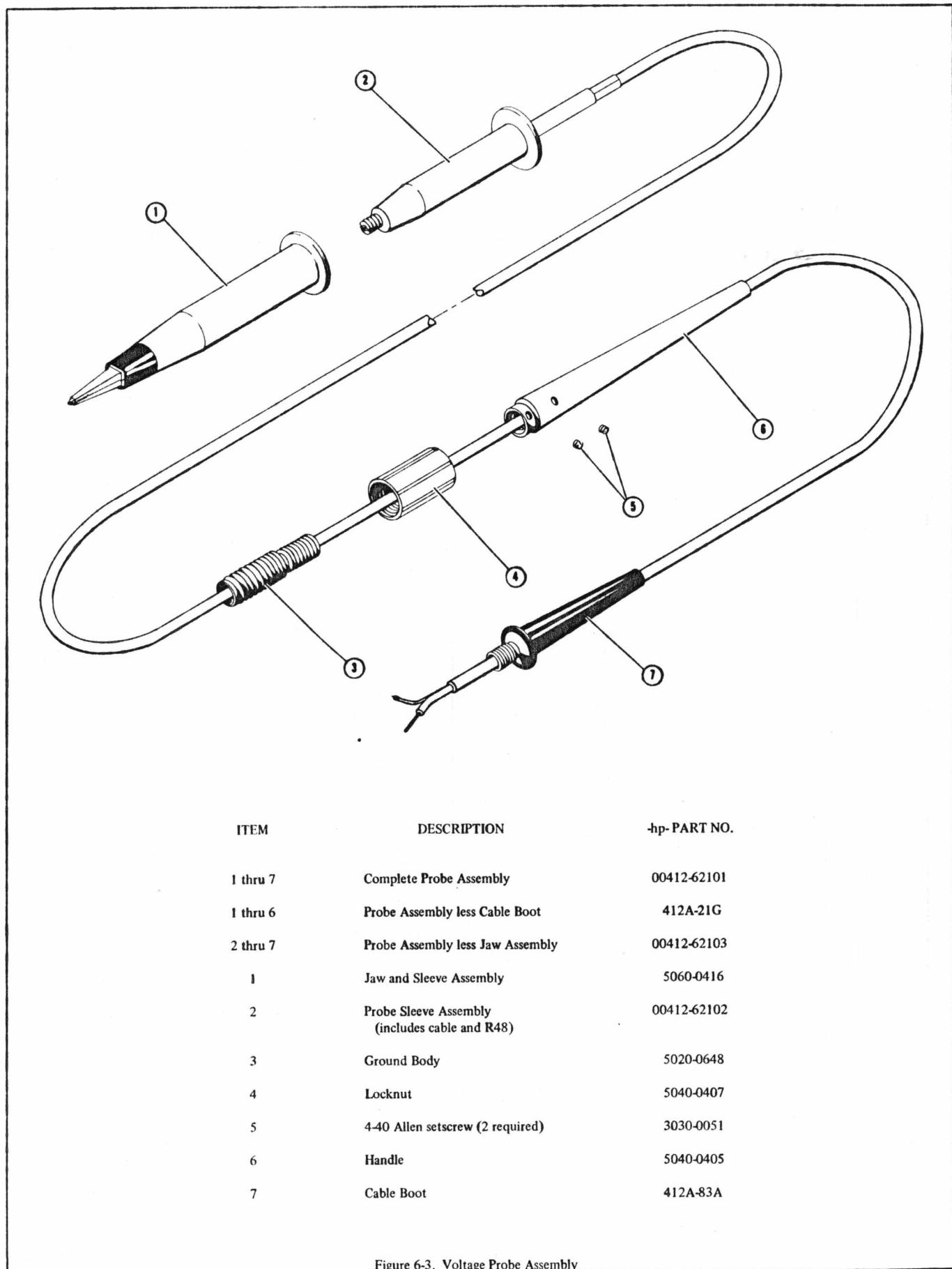
Figure 6-3. Voltage Probe Assembly
