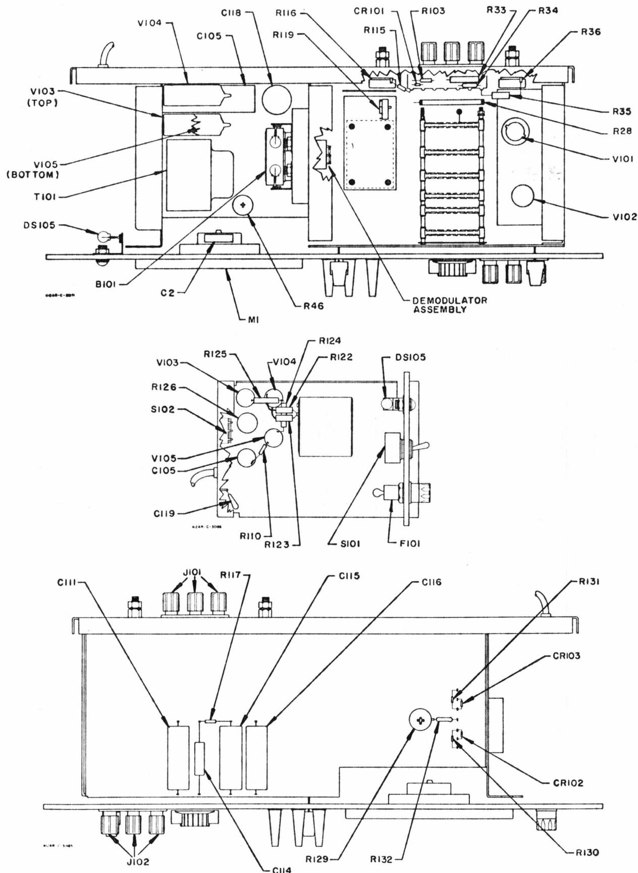
Figure 7-2. Location of Chassis Mounted Parts, Rack Model
