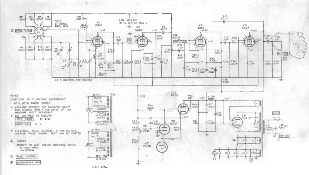
SCHEMATIC DIAGRAM OF MODEL 200H SERIAL 613 & ABOVE
