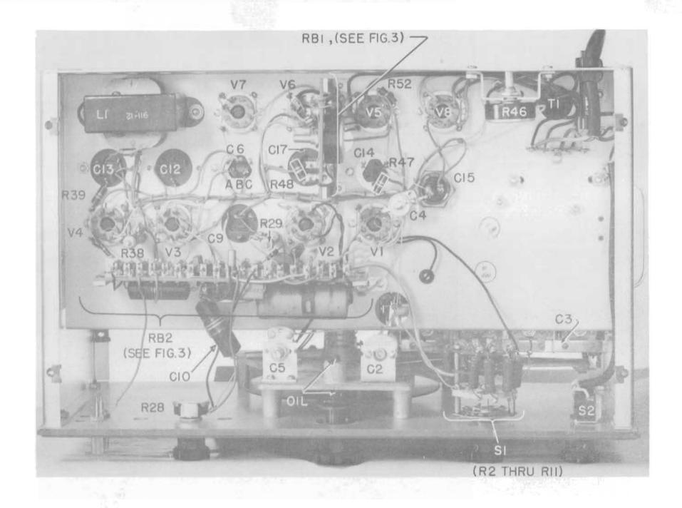
Fig. 2. Model 200H Bottom View Bottom Plate Removed
