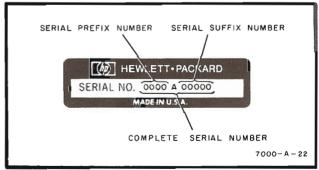
Figure 1-2. Instrument Serial Number
