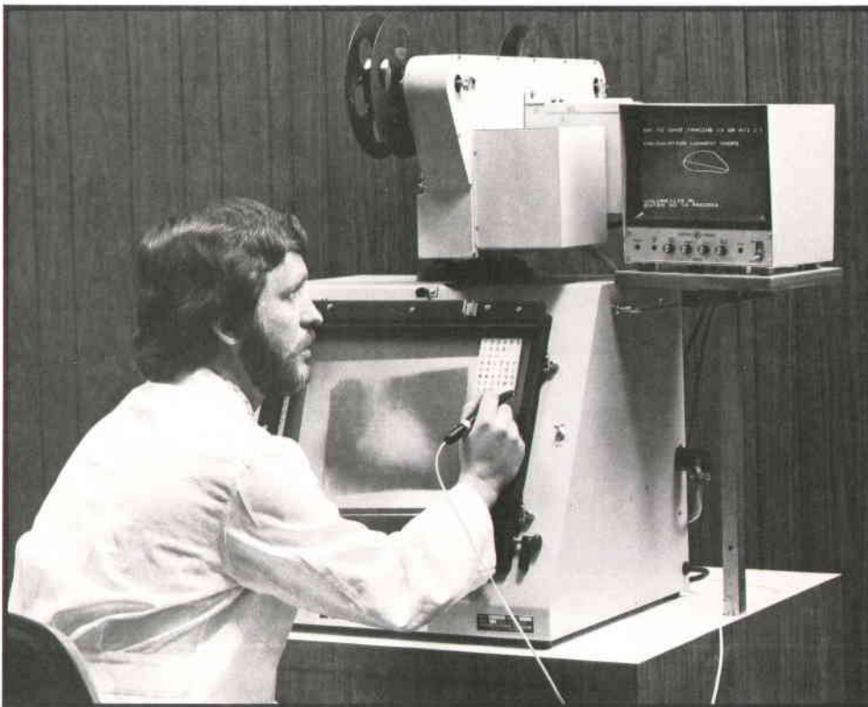
Fig. 4. Angio-analyzer uses a cineprojector and a rear-projection screen with a front-viewing surface that eliminates parallax errors. The position digitizer has a linear microphone along the top edge of the screen and another along the left edge; it measures the times taken for ultrasound pulses to travel from the pen to each microphone, from which the computer calculates distance. The position of the symbols on the "keyboard" are interpreted as symbols by the computer.
