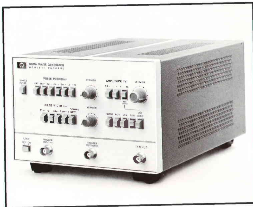
Fig. 1. Model 8011A Pulse Generator produces 16-volt pulses at repetition rates up to 20 MHz. It has convenient pushbutton operation.
