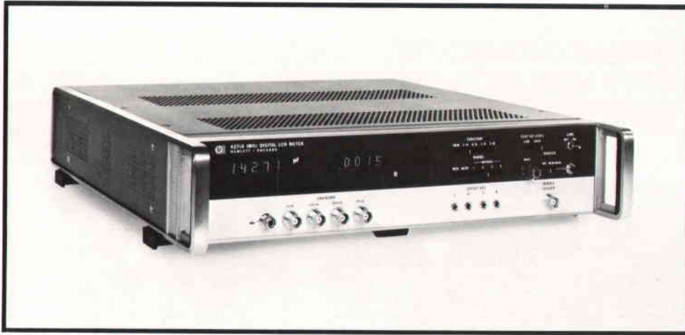
Fig. 1. Model 4271A LCR Meter has a four-digit display with 90% overrange. Basic accuracies are \pm 0.1\% in C measurements and \pm 0.2\% in L, R, and G measurements. It also measures dissipation factors. All measurements are made at 1 MHz and at very low test signal levels.
