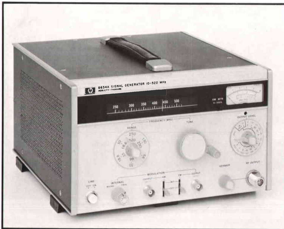
Fig. 1. Model 8654A is a compact, low-cost, solid-state signal generator that provides automatically leveled power from +10 to -130 dBm over a frequency range of 10 to 520 MHz. Amplitude and frequency modulation are independent and can be internal or external.
