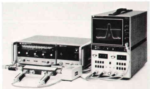
Model 8755L Frequency Response Test Set uses the logarithmic amplifier described here.
