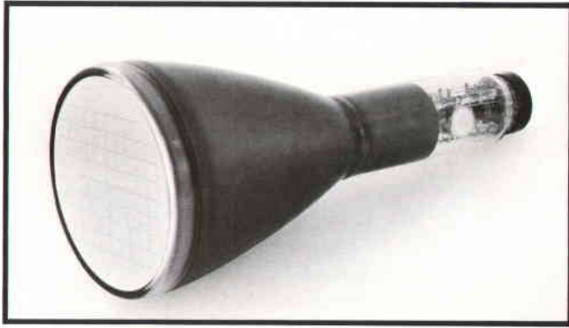
Fig. 5. The cathode-ray tube for the new oscilloscopes uses an uncomplicated structure that reduces the number of manufacturing steps.
