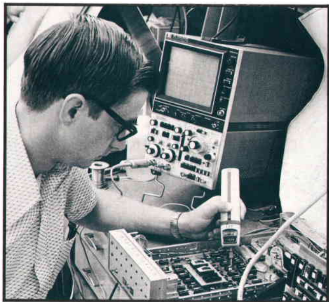
Fig. 2. Slide switch adjacent to the display inverts the numerals so readings can be taken with the probe upside down.
