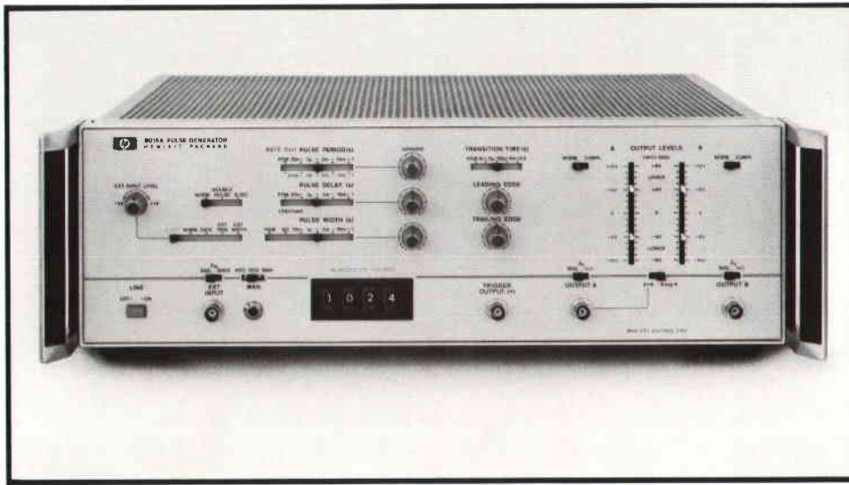
Fig. 3. Output levels are set by calibrated linear controls. The upper slider sets the upper pulse excursion and the lower slider establishes the lower excursion. The center scale is used when Z_s switches are set to 50\Omega while driving 50\Omega loads. The outside scales are used when driving either high-impedance loads with Z_s set to 50\Omega , or a 50\Omega load with Z_s set to 1k\Omega . Controls provide visual indication of compatible settings. As long as the PULSE DELAY and WIDTH controls are to the left of the PULSE PERIOD control, there is no danger that the width or delay settings would exceed the pulse period.
