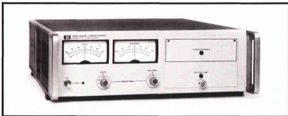
Fig. 1. Model 6140A Digitally-Programmable Current Source supplies current accurately at levels up to \pm 160 mA in response to digital input commands. It accepts various logic levels and formats according to interface circuit boards that are installed through the removable panel on the front-panel.
