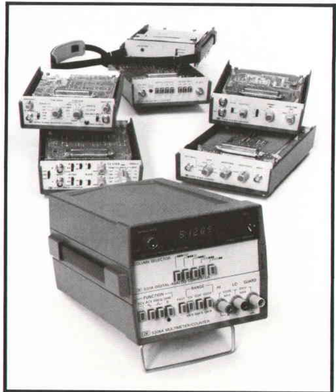
Fig. 1. Two new modules for the 5300 Measuring System are Model 5306A Multimeter/Counter (bottom module of instrument in foreground) and Model 5311A Digital-to-Analog Converter (center module). The Multimeter/Counter measures dc voltage, ac voltage, resistance, and frequency. Other elements of the system are the mainframe (top module), four counter/timer modules and a battery pack.
