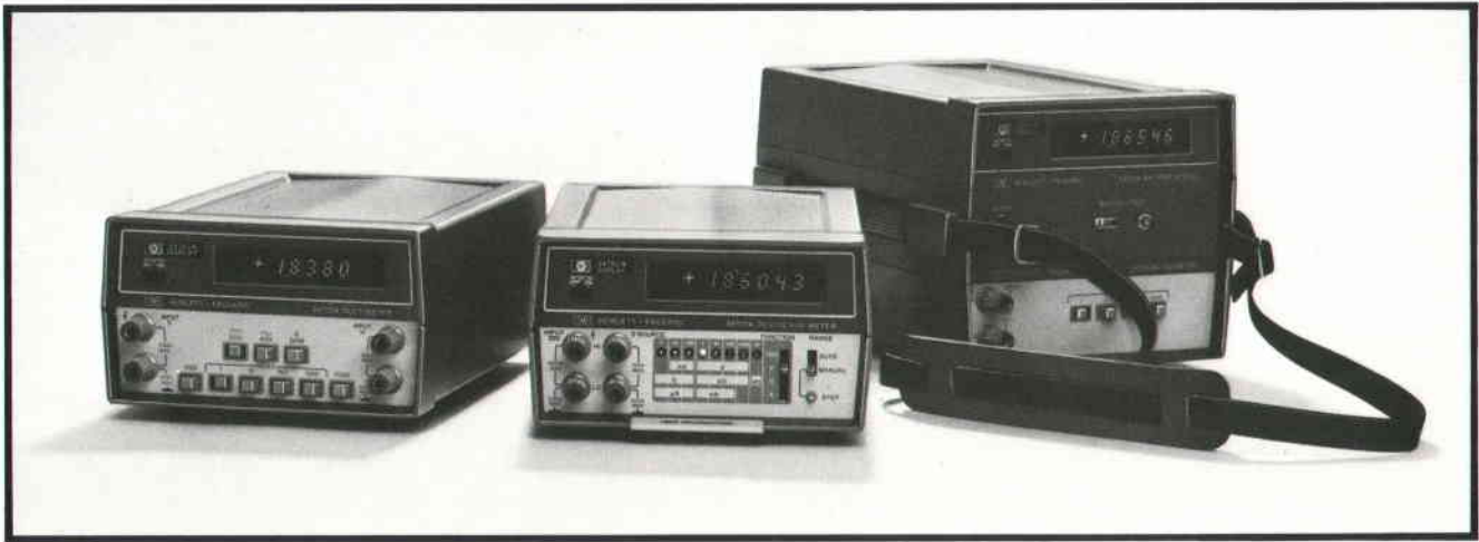
Fig. 1. New modules for Model 3470 Measurement System, shown in center, give 5-digit resolution, higher sensitivity, autoranging and self test. Modules are compatible with units announced earlier so wider range of multimeter configurations, three of which are shown here, can be formed to meet various measurement requirements.
