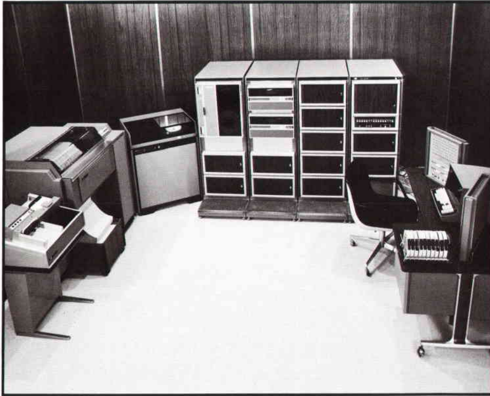
Fig. 1. HP 3000 Computer System has multilingual and multiprogramming capabilities usually found on much larger systems.
