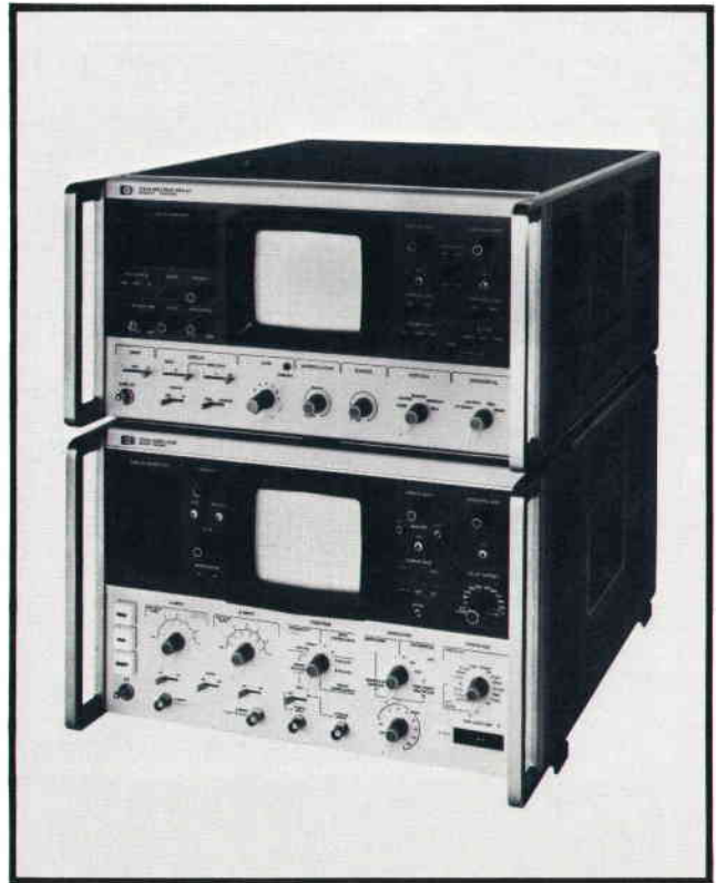
Fig. 1. New Model 3720A Spectrum Display (top) complements 3721A Correlator (bottom). Spectrum Display accepts correlation functions computed by Correlator and transforms them into the frequency domain, computing real and imaginary coefficients at 100 different frequencies.
