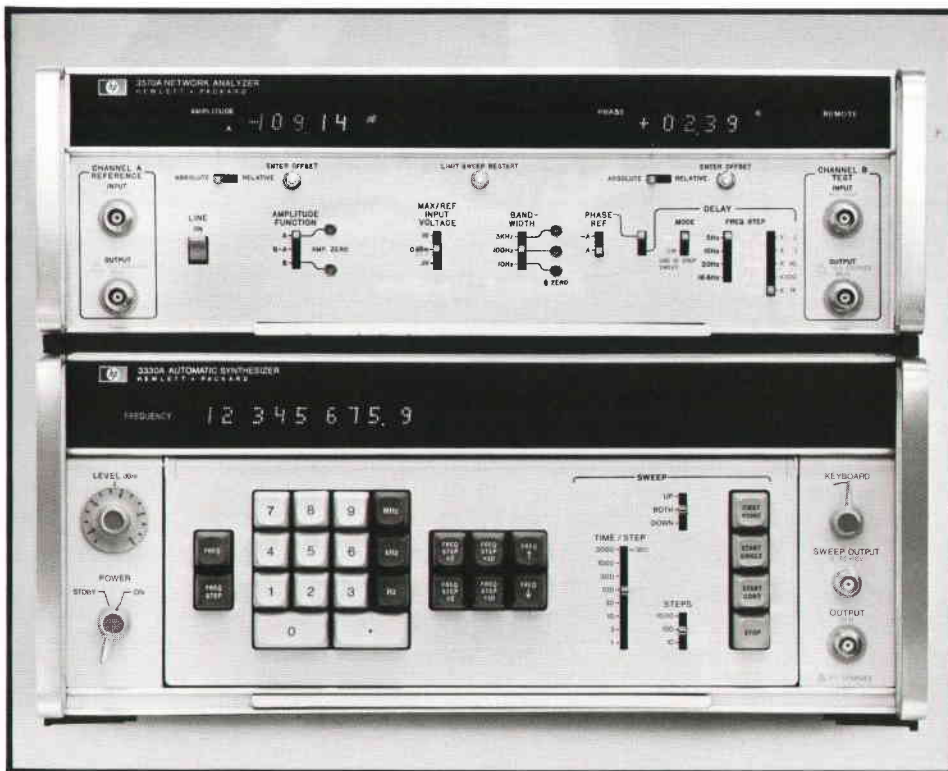
Fig. 1. Model 3570A Network Analyzer (upper unit) functions as two-channel tracking detector with one of HP's 0-13 MHz Frequency Synthesizers (lower unit) to form complete network analysis system. Network Analyzer shown here has Delay / Limit Test / Offset option.
