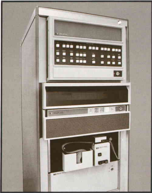
Fig. 1. Model 7900A Disc Drive operates in environments too severe for other drives. It's also fast for a small moving-head drive: average seek time is 30 ms, average latency is 12.5 ms. Data transfer rate is 312,000 bytes per second. Capacity on one fixed disc and one removable cartridge is 5 million 8-bit bytes.
