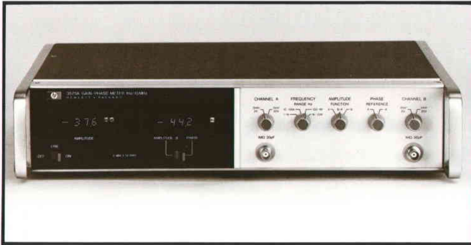
Fig. 1. New HP Model 3575A Gain-Phase Meter measures amplitude ratio and phase difference between two signals in 1 Hz–13 MHz frequency range. Optional version shown here has two digital readouts. Standard version has left readout only and switch selects gain or phase for display. Other options provide for external digital control and readout of all functions for systems use.
