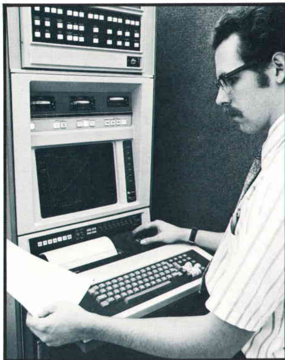
Fig. 1. Model 8500A System Console is designed specifically for use with automatic measurement systems. The complete console is contained in one rack, which also has space for the system computer.
