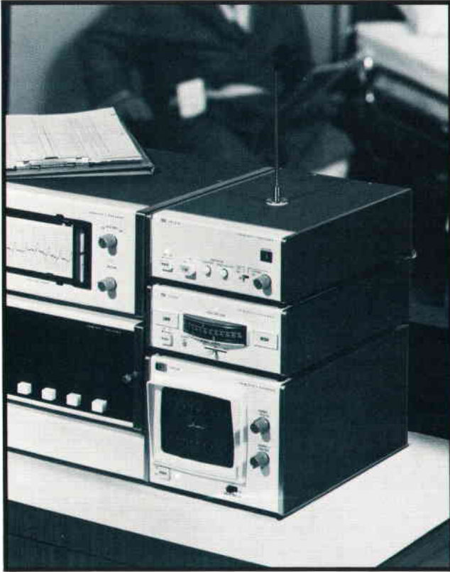
Fig. 2. Telemetry Receiver conforms to modular design of HP patient-monitoring instruments. Modular approach makes it possible to configure monitoring systems using the telemetry link to meet the particular requirements of any hospital.
