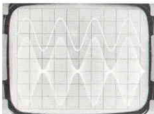
Modulation distortion characteristics. 20-MHz carrier with AM >90% at a 2-kHz rate. Carrier and detected envelope shown.
