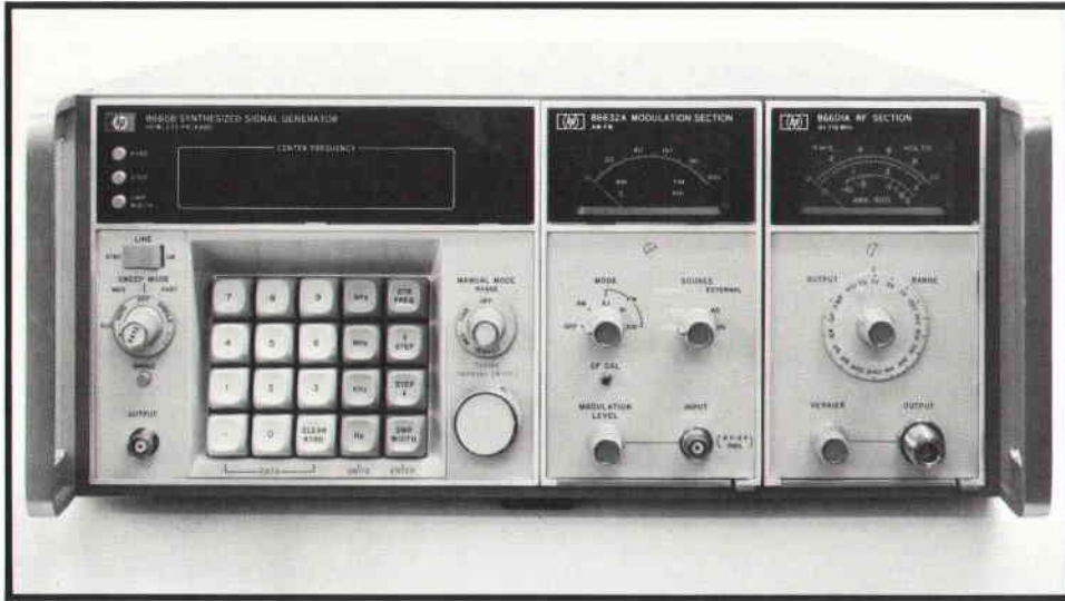
Fig. 2. Complete instrument with 8660B keyboard-controlled synthesized generator, 86601A 110-MHz rf section, and 86632A modulation section.
