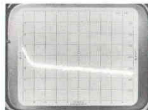
Phase noise in a 1-Hz band (SSB) referenced to carrier. Reference (top graticule line) is -70 dB (20 kHz/cm, carrier = 30 MHz).
