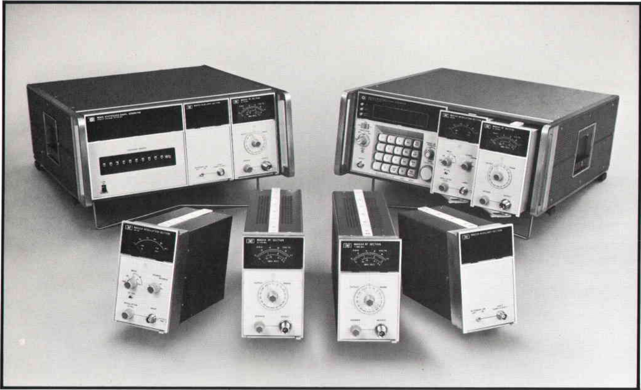
Fig. 1. The 8660 system poses for a family portrait. 8660A (left rear), 8660B (right rear), are basic mainframes. Modulation facilities are added with 86632A Modulation Section (near left) in central plug-in position, or 86631A Auxiliary Section (near right) is substituted. Near center pair of plug-ins are RF Sections, 86601A for 0.01-110 MHz, 86602A for 1-1300 MHz.
