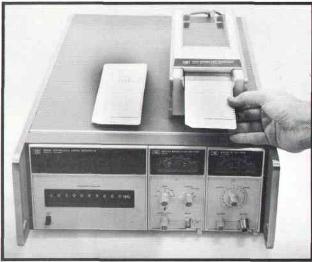
Fig. 11. Synthesizer can be programmed with Model 3260A Marked Card reader.
