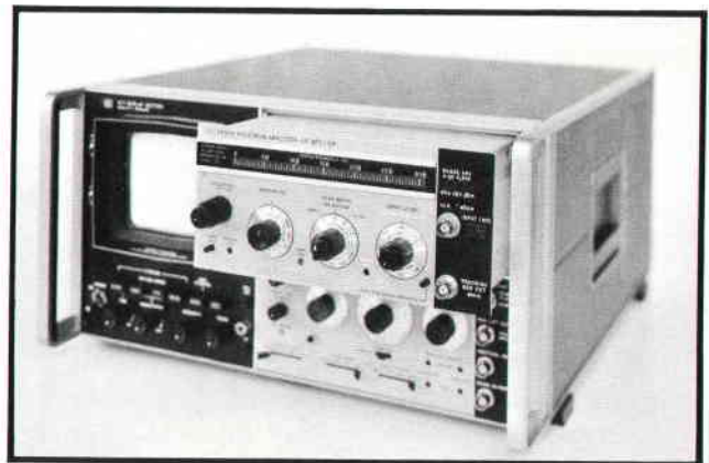
Fig. 1. A new plug-in LF Section for the HP Spectrum Analyzer family to 300 kHz, features built-in tracking generator and crystal markers. A low-noise isolated front end provides high sensitivity (20 nanovolts) and freedom from ground-loop pickup. Absolute calibration in power for several impedances is provided, with an option for balanced input.
