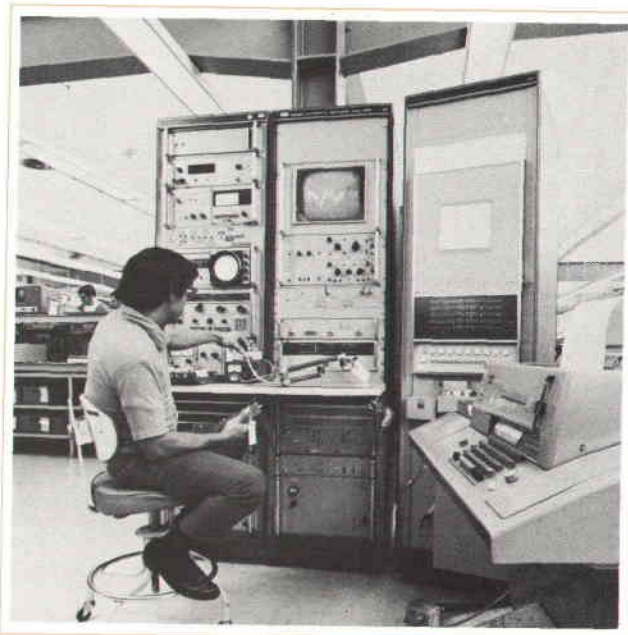
Fig. 3. Each attenuator undergoes tests for residual loss, reflection coefficient, and attenuation at each of a large number of frequencies from dc to 18 GHz. The full set of tests takes about 12 minutes on especially modified HP Model 8542 Automatic Network Analyzer equipment.
