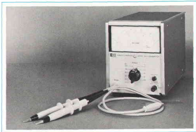
Fig. 1. This Hewlett-Packard Model 4328A Milliohmmeter measures low resistances from 1 milliohm to 100 ohms full scale with a resolution of 20 \mu ohms.
