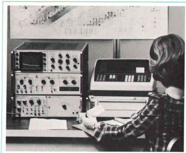
Fig. 3. HP 5403A MCA/Calculator System consists of analyzer, coupler/controller, and calculator. This system is capable of a higher degree of automation than the minimal analyzer/calculator system. The two-way coupler permits calculator control of analyzer functions as well as transfers of data among the analyzer, the calculator, and peripheral devices.
