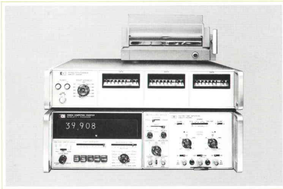
Fig. 1. New HP 5376A Programmer (center) is a programming and interface device for the HP 5360A Computing Counter. Together the two instruments are the nucleus of a class of low-cost programmable systems with built-in computer capability. Punched-card reader (top) provides optional programming method.
