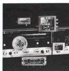
Cover: The rf elements are all-microcircuit in the solid-state microwave sweeper to which this entire issue is devoted. Shown in front of the sweeper on our cover (left to right and top to bottom): the directional detector, the frequency converter module, the 2-4 GHz YIG oscillator, the PIN absorptive modulator, and the 0.1-2 GHz amplifier.
