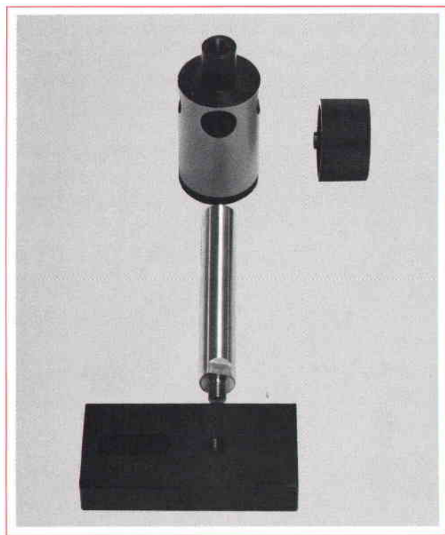
Fig. 3. Reflector, or 'cube corner', is designed for easy mounting in a variety of ways, and for easy alignment. Turning a single knurled ring clamps all axes.
