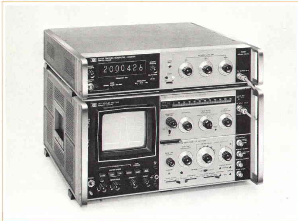
Fig. 1. Combination Tracking Generator and Counter (above) mates with Spectrum Analyzer (below) to form powerful swept measuring system.
