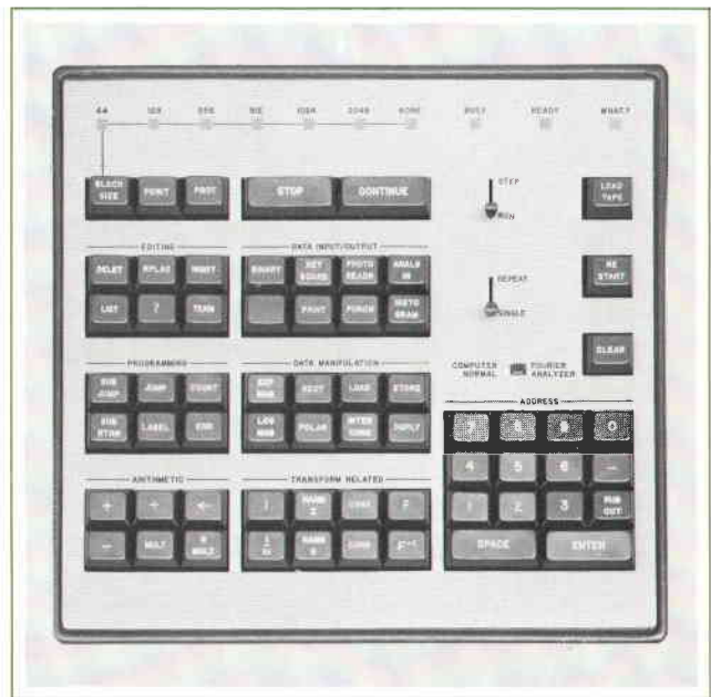
Fig. 2. All Fourier analyzer operations are keyboard controlled. The principal operations—Fourier transforms, convolution, correlation, complex multiplication, coordinate transformations, and so on—can be called for by single keystrokes, or strung together using the programming and editing features to form routines to be run automatically later on. Typical routines can change the analyzer into a spectrum analyzer, a correlator, an averager, and many other instruments.
