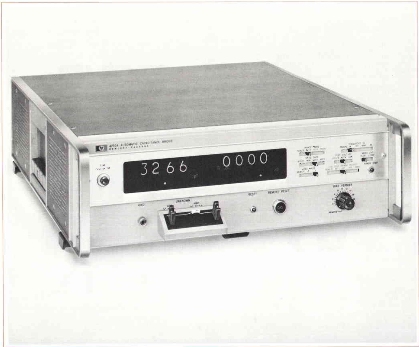
Fig. 1. The new HP Model 4270A Automatic Capacitance Bridge can measure grounded cables and input capacitance of amplifiers with the LOW terminal grounded. In L-GROUND operation, the instrument still retains the guarded feature.
