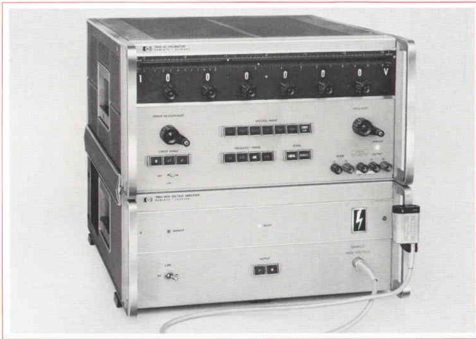
Fig. 1. Combining the Model 746A High Voltage Amplifier (lower unit) with the Model 745A AC Calibrator makes available ac calibration voltages to 1100 V in one instrument.
