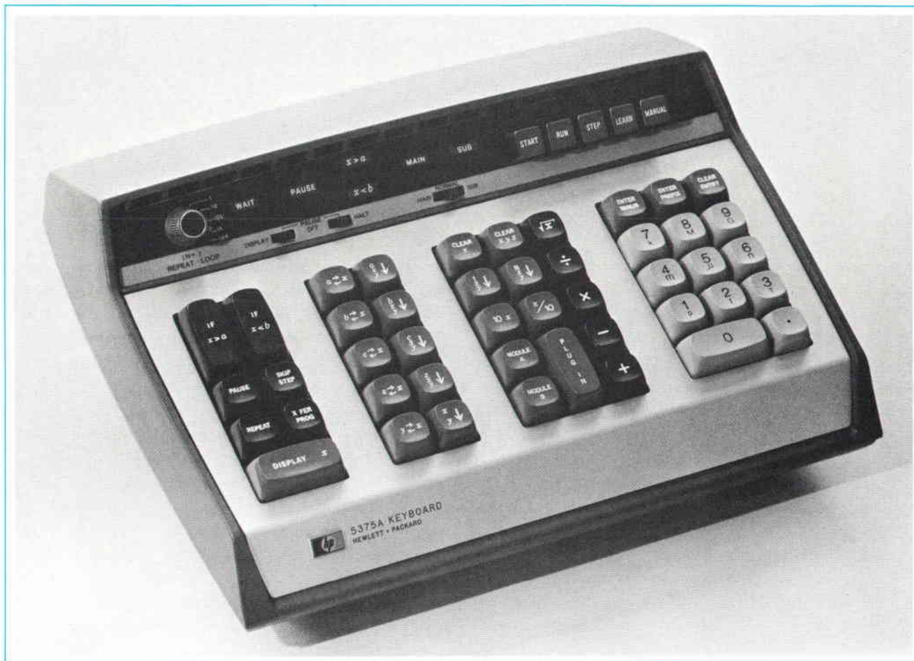
Fig. 1. Model 5375A Keyboard is an external programmer for Model 5360A Computing Counter. Programs can be executed manually, or learned and executed repetitively. The Keyboard can make comparisons, do program looping and branching, and insert constants into programs.
