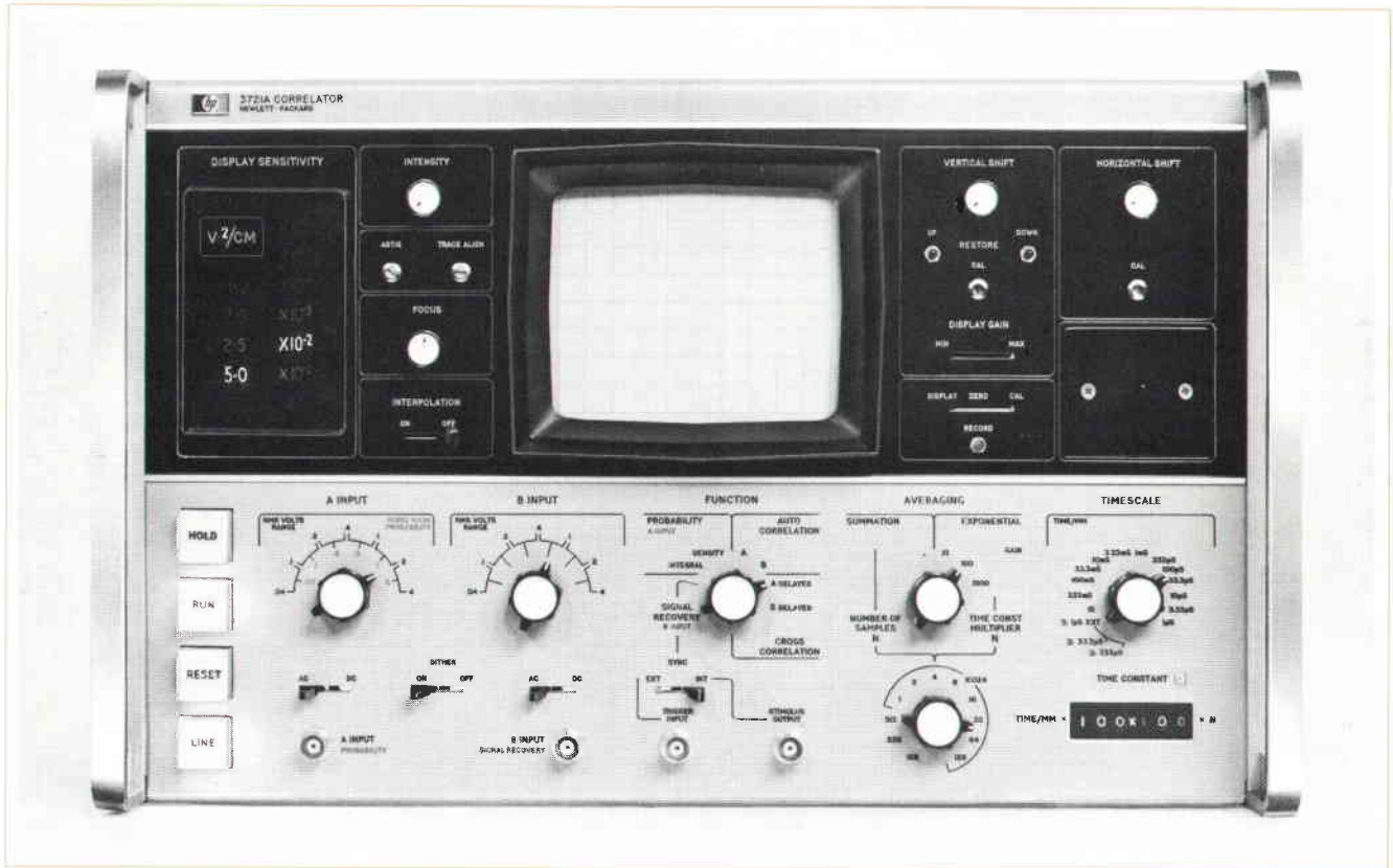
Fig. 1. Despite its versatility, Model 3721A Correlator is as easy to use as an oscilloscope. An illuminated panel shows the display sensitivity in V^2/cm for correlation and in V/cm for signal averaging (signal recovery). The correlator has a wide selection of measurement parameters and modes of operation, including a 'quick-look' mode which minimizes delays in setting up experiments.
