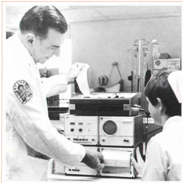
Fig. 2. Arrhythmia Monitor (unit left of oscilloscope monitor) is in compact cabinet that matches other units in Hewlett-Packard Patient Monitor systems.
