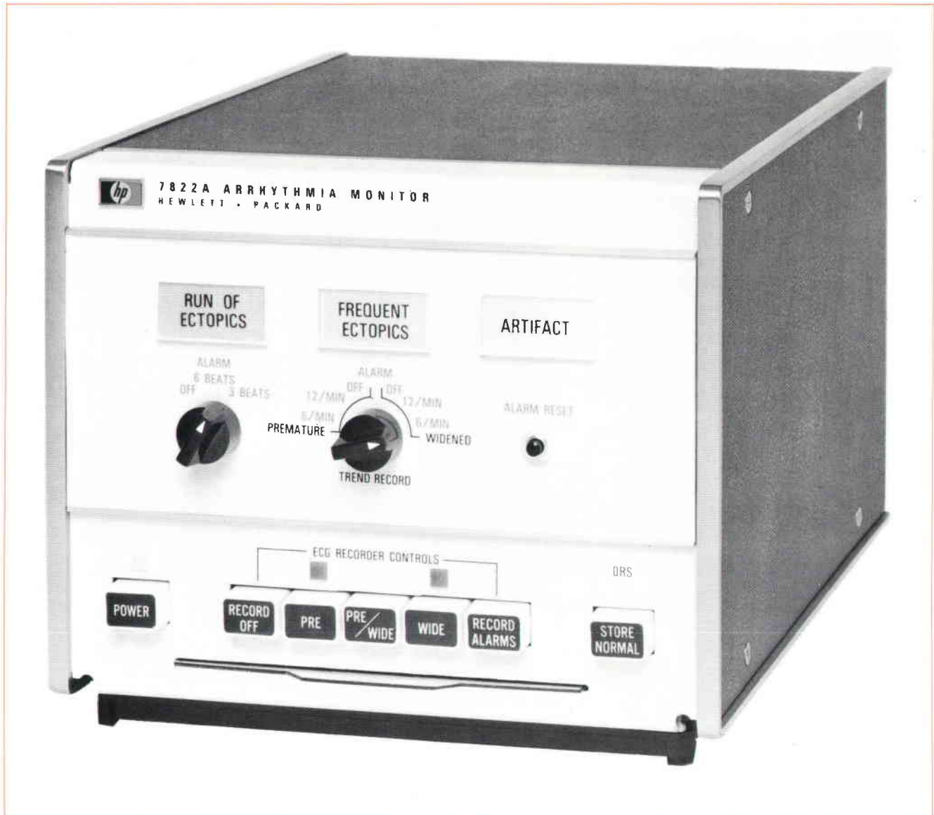
Fig. 5. Arrhythmia Monitor detects every premature and every widened beat, flashing appropriate indicator lamp (just above row of pushbuttons). Five pushbuttons at lower center select type of beat to be recorded on electrocardiograph. Upper controls select alarm criteria (see Fig. 11).
