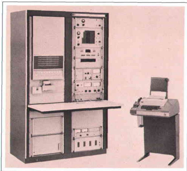
Fig. 1. HP Model 9500A is a typical computer-controlled, modular, multipurpose test system. It stimulates the unit under test and measures its responses, then processes and records the data. Stimuli available are dc, low-frequency ac (to 100 kHz), and high-frequency ac (to 500 MHz).
