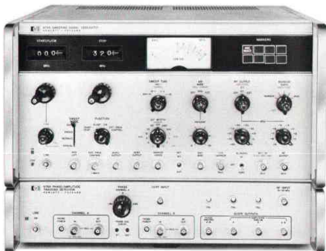
Fig. 1. This new HP Model 675A/676A is a low-frequency network analyzer covering the range from 10 kHz to 32 MHz.
