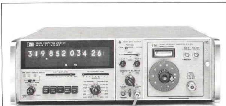
Fig. 1. Model 5360A Computing Counter is orders of magnitude more powerful than earlier counters. It measures CW or pulsed carrier frequencies between 0.01 Hz and 320 MHz to as many as 11 significant digits. Frequency-converter plug-ins extend its range to 18 GHz. It measures period (and time interval with another plug-in) with 1 ns accuracy and 0.1 ns resolution.
