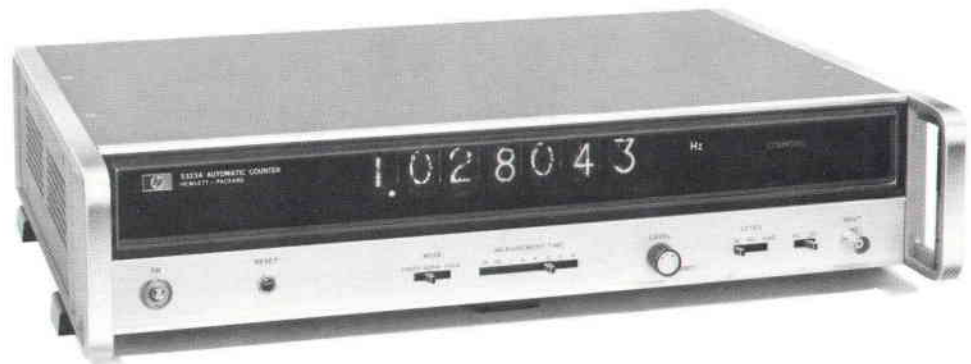
Fig. 1. Model 5323A Automatic Counter measures frequencies by measuring and inverting the period of the input signal. It's completely automatic — the only function control is for selecting the measurement time, which can have non-decade or even (using an external gate) unknown values. Resolution is 7 digits maximum for any frequency, 0.125 Hz to 20 MHz.
